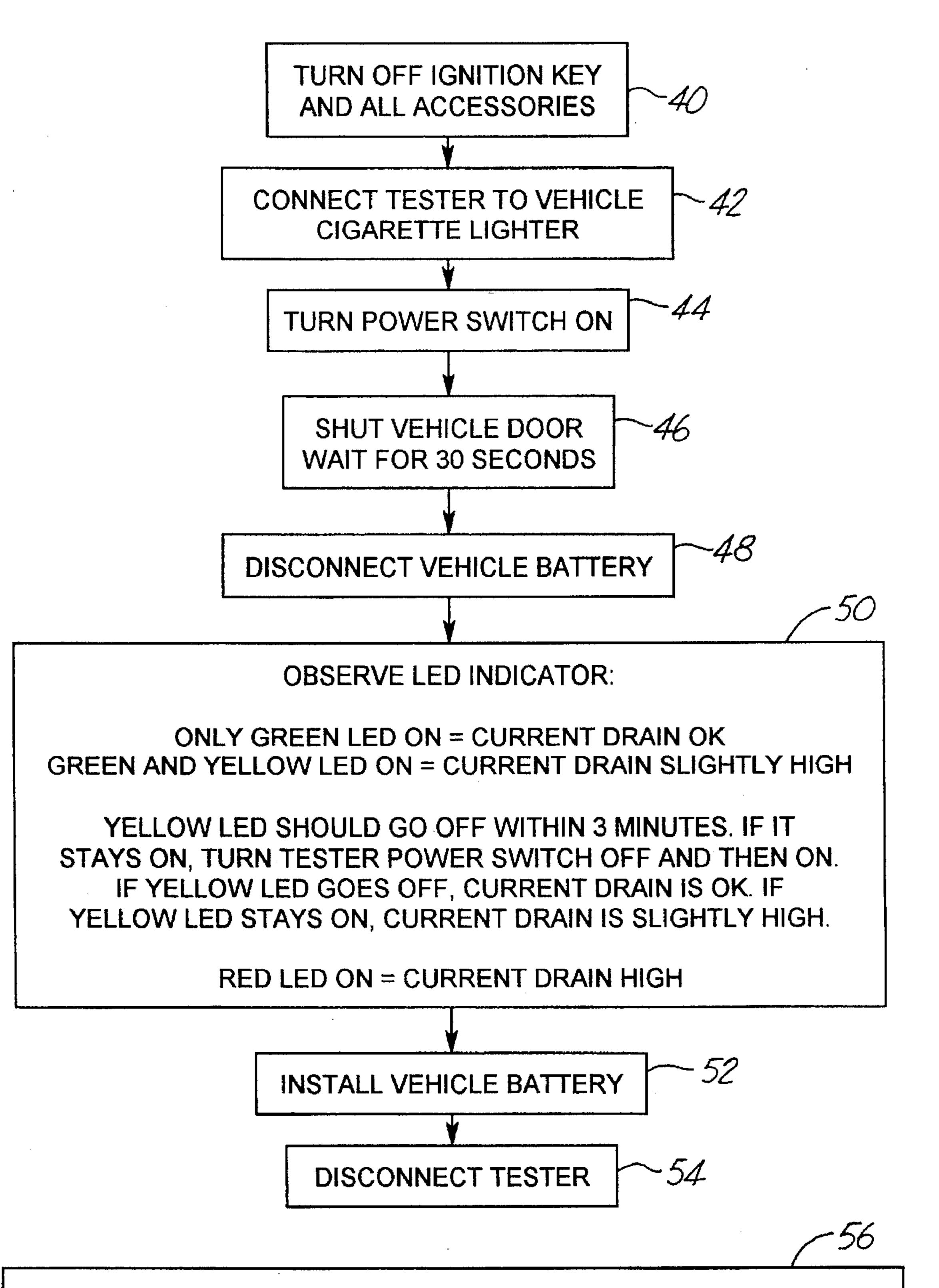
NOTE: DUE TO SHORT CIRCUIT CONDITION OR OVER CURRENT CONDITION, IF THE BEEPER GOES ON, CORRECT THE FAULT AND TURN THE POWER SWITCH OFF AND THEN ON.
