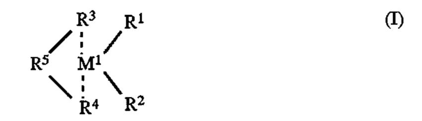
in which M<sup>1</sup> is titanium, zirconium, hafnium, vanadium, niobium or tantalum and an aluminoxane. This copolymer has a very high molecular weight, a very narrow molecular weight distribution, very high syndiotaxicity, advantageously low melting points and rubber-like behavior. Molded articles produced from the polymer are distinguished by high transparency, flexibility and tear strength. Their main areas of application are packagings of any type.
