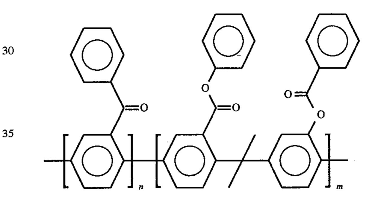
A solution: of parapolybenzoylphenylene (0.5 g; 2.8 mmol of monomer units) in 50 ml of methylene chloride is treated with 0.1 g (0.29 mmol) of 50% 3-chloroperoxybenzoic acid (MCPBA) and refluxed for 7 days. This mixture is poured into acetone to precipitate the product. Approximately 10% of the sidechain appendages of the resulting rigid-rod copolymer contain reactive ester groups.
