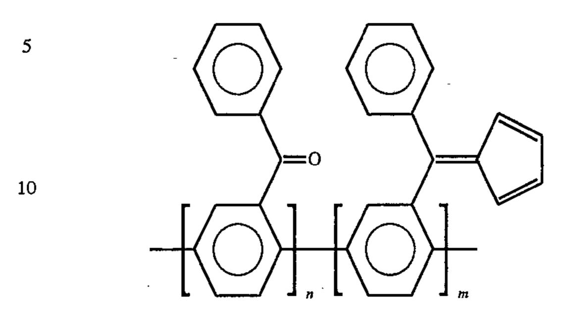
A solution of parapolybenzoylphenylene (1.0 g; 5.6 mmol of monomer units) in 100 ml of diphenyl ether is treated with 0.25 ml (0.5 mmol) of 2 molar sodium cyclopentadienide (tetrahydrofuran solution) and heated at 100° C. for 4 hours. This mixture is poured into 1 molar hydrochloric acid in ethanol to precipitate the product. Approximately 9% of the sidechain appendages of the resulting rigid-rod copolymer contain reactive fulvene groups.
