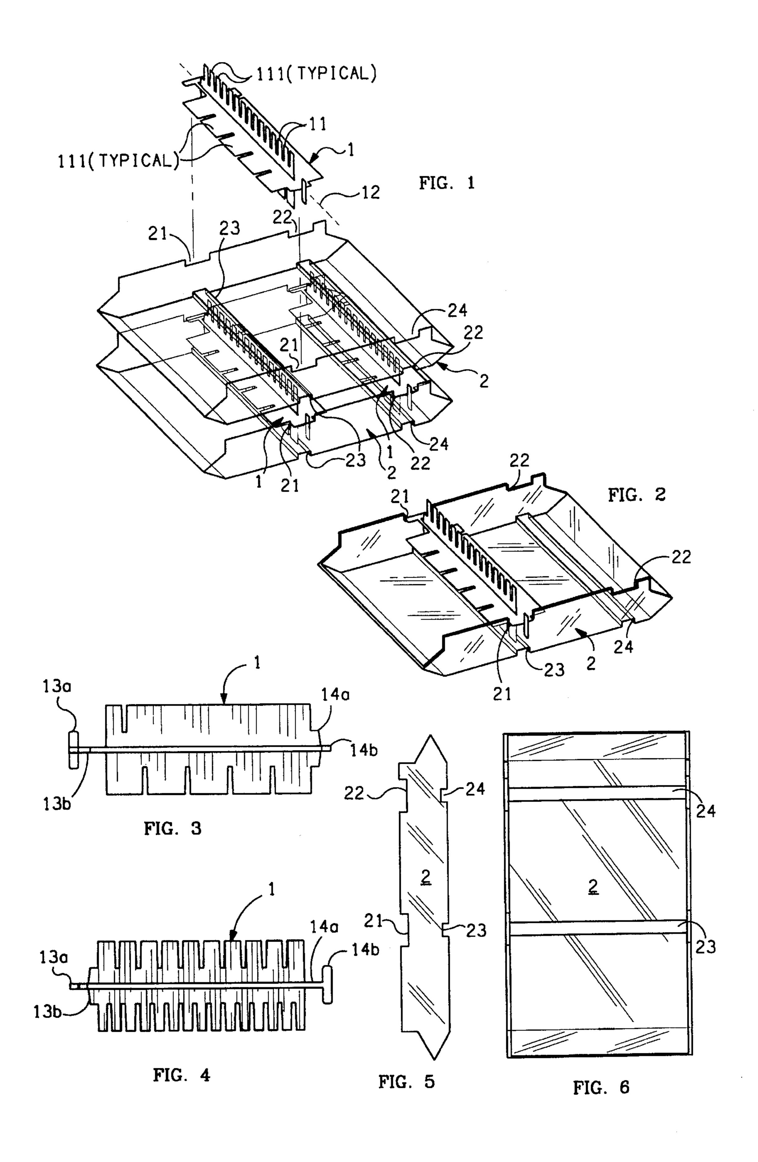
COMB ELEMENTS ROTATING IN POSITION TO PLACE SELECTED SLIT ARRAYS IN THE GEL OF AN ELECTROPHORESIS AGAROSE GEL TRAY, PARTICULARLY AS ALSO SERVE AS SPACERS BETWEEN STACKED TRAYS
