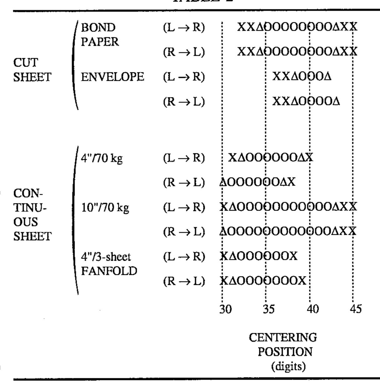
Table 2 discloses a non-exhaustive list of paper types available including cut sheets such as bond paper and envelopes or continuous sheets, such as a 4"/70 kg type, 10"/70 kg type, 4"/3-sheet fanfold type, and the like. Therefore, the aforementioned sheet forward start carriage position C4 is determined for every type of sheet (i.e., whether
