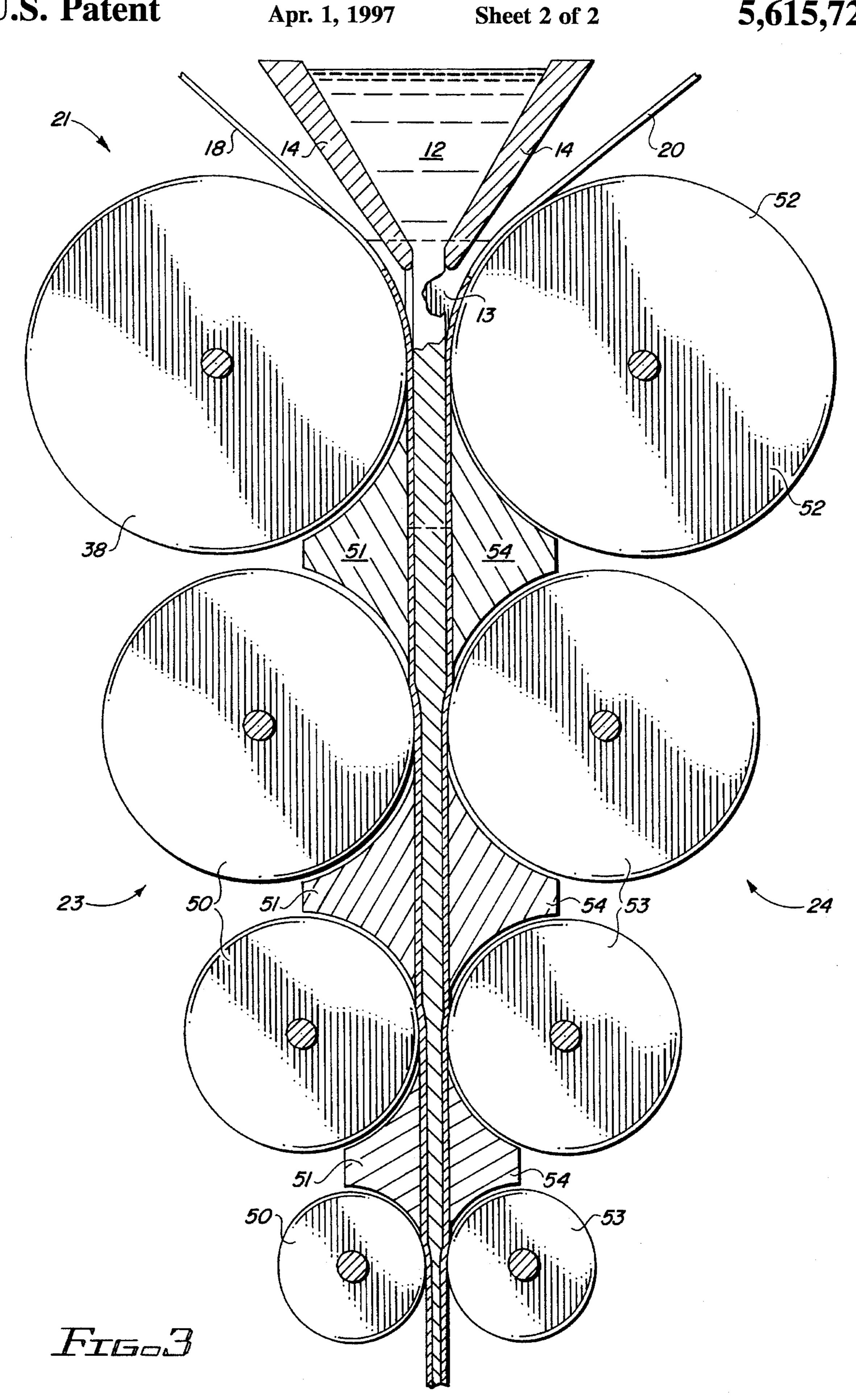
This invention relates generally to composite metal strips and sheets and to methods and apparatus for making the 5 same. More particularly, the invention concerns casting molten metal between two adjacent moving cold-rolled strips of metal and fusing said metal and said strips to form a composite structure. In optimal practice, a light metal coating may be applied to one or both sides of the composite 10 metal member.
