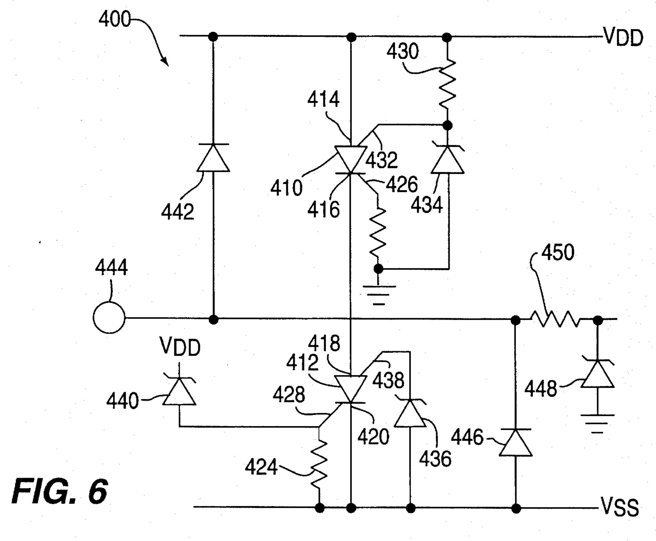
The invention is directed to an electrostatic (ESD) protection circuit for an integrated circuit (IC), and, more particularly to an ESD protection circuit for the power supply and input/output (I/O) connections of a low voltage submicrometer IC.
