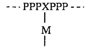
where P represents a repeating polymer chain unit, M represents the maleic moiety, and X is the polymer unit to which M is bonded.
