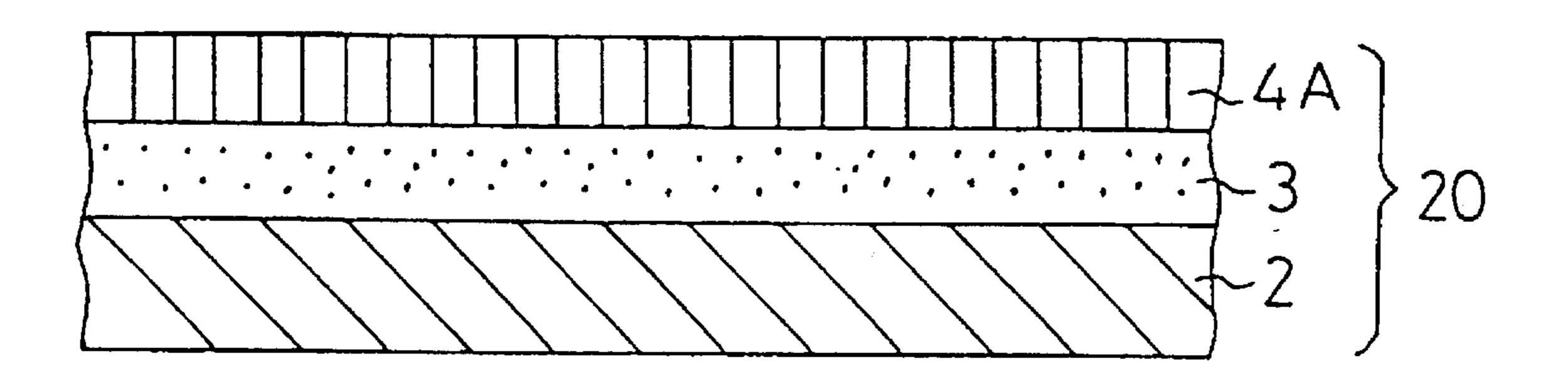
IMAGE TRANSFER SHEET COMPRISING AN INTERMEDIATE LAYER AND AN IMAGING LAYER WHEREIN THE POLYMER IN THE INTERMEDIATE LAYER AND THE IMAGING LAYER HAVE A COMMON MONOMER
