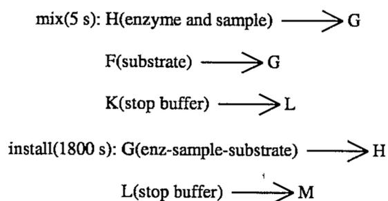
At the conclusion of this step (e) the assay solution present in the reading chamber has incubated 30 minutes and now contains the ALAD/ALA reaction product porphobilinogen.
