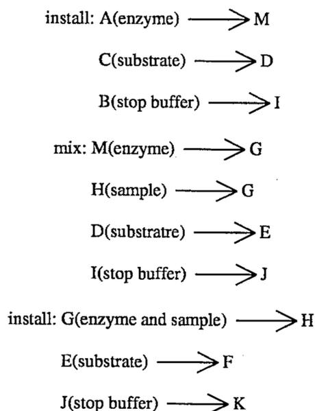
Thus, at the end of the mix-install cycle performed in this step (c), the enzyme solution has been mixed with the original sample and is now present in the reading chamber H along with the sample; the substrate solution has not yet combined with the enzyme sample mixture but is now positioned in region F; and the stop buffer has been moved to region K.
