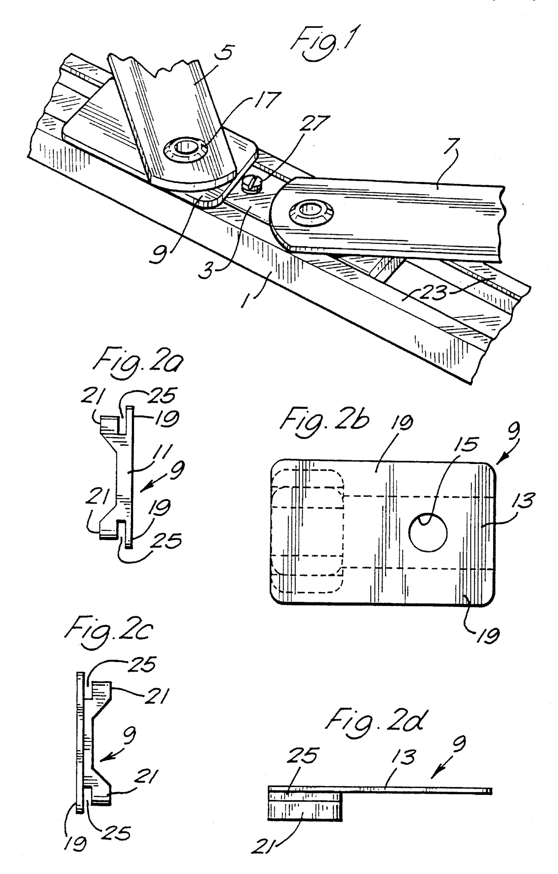
This invention relates to frictions stays, and in particular to an anti-rubbing block for a friction stay.
