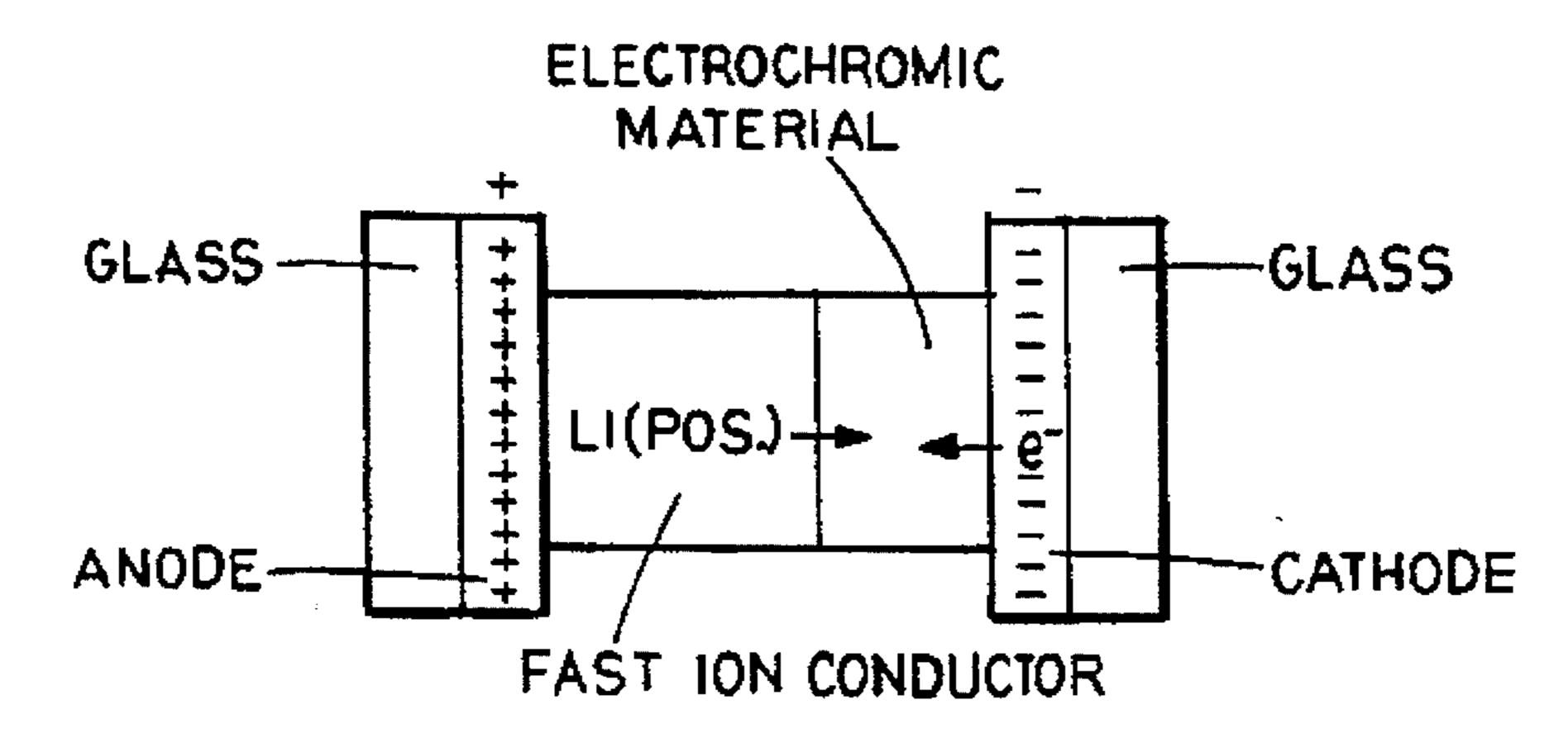
REDUCTION - GAIN OF ELECTRONS LI(POS) AND e<sup>-</sup> (NEG.) INCLUSION OR LI(NEG) AND HOLE EXTRACTION
