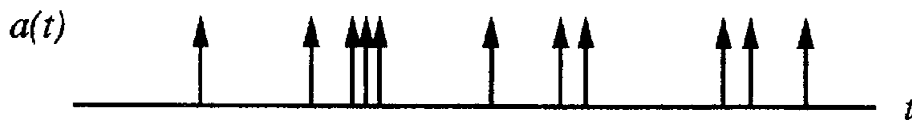
Figure 2: A generic traffic stream described by a train of impulses.
