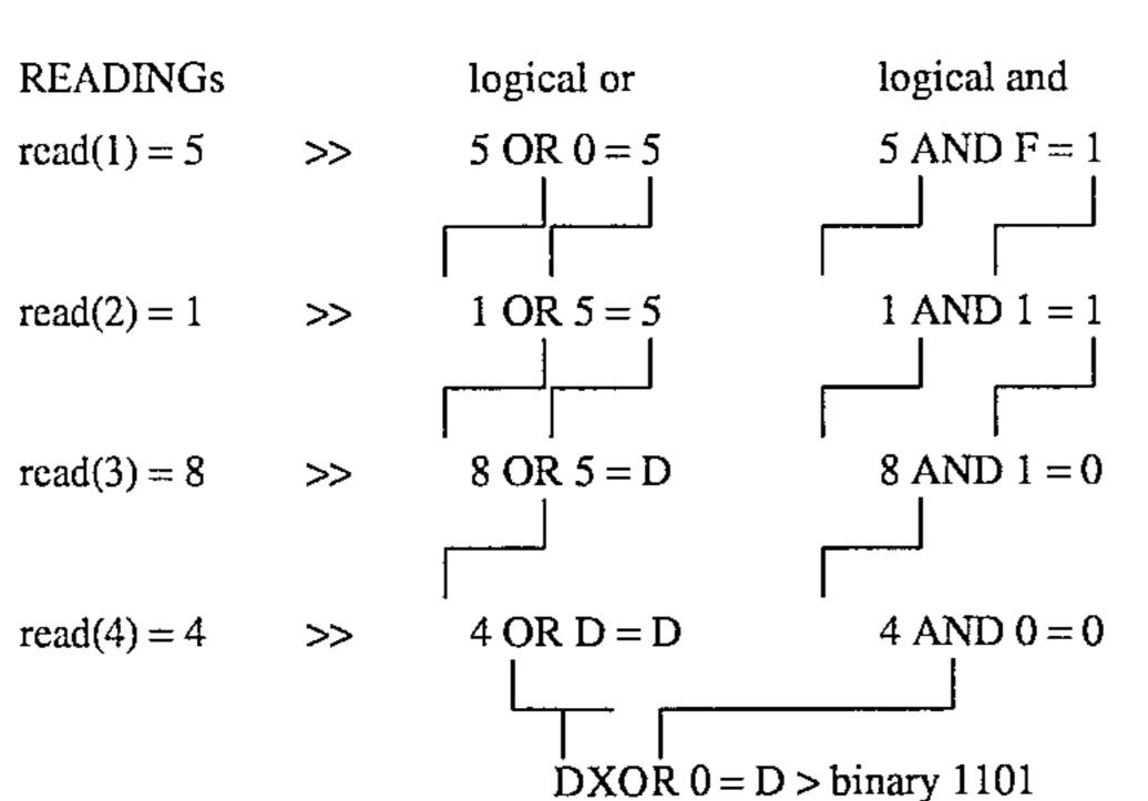
Example 1 illustrates the operation of the logical OR gates and logical AND gates. The four successive readings are hexadecimal 5, hexadecimal 1, and hexadecimal 8, and hexadecimal 4.
