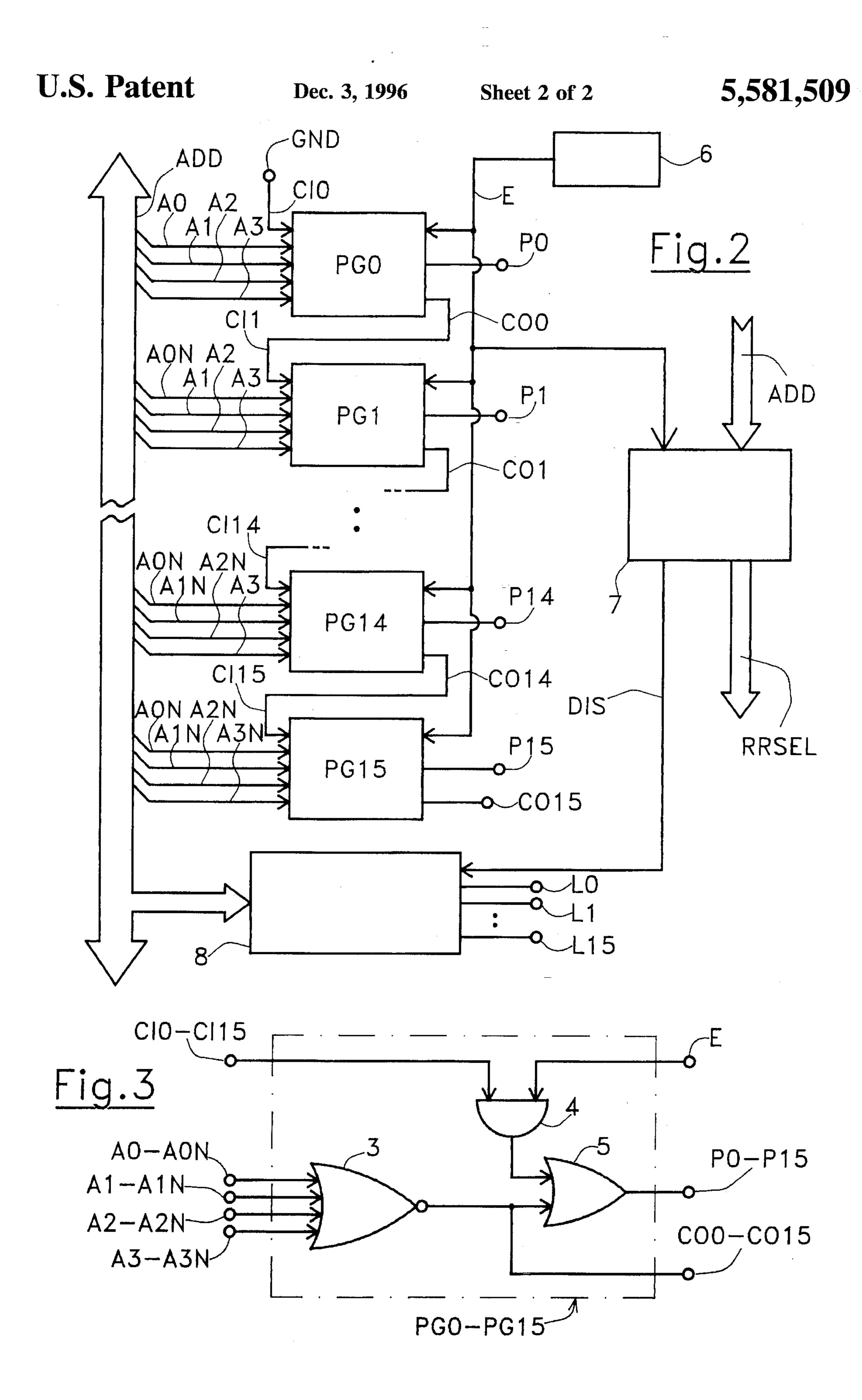
DOUBLE-ROW ADDRESS DECODING AND SELECTION CIRCUITRY FOR AN ELECTRICALLY ERASABLE AND PROGRAMMABLE NON-VOLATILE MEMORY DEVICE WITH REDUNDANCY, PARTICULARLY FOR FLASH EEPROM DEVICES
