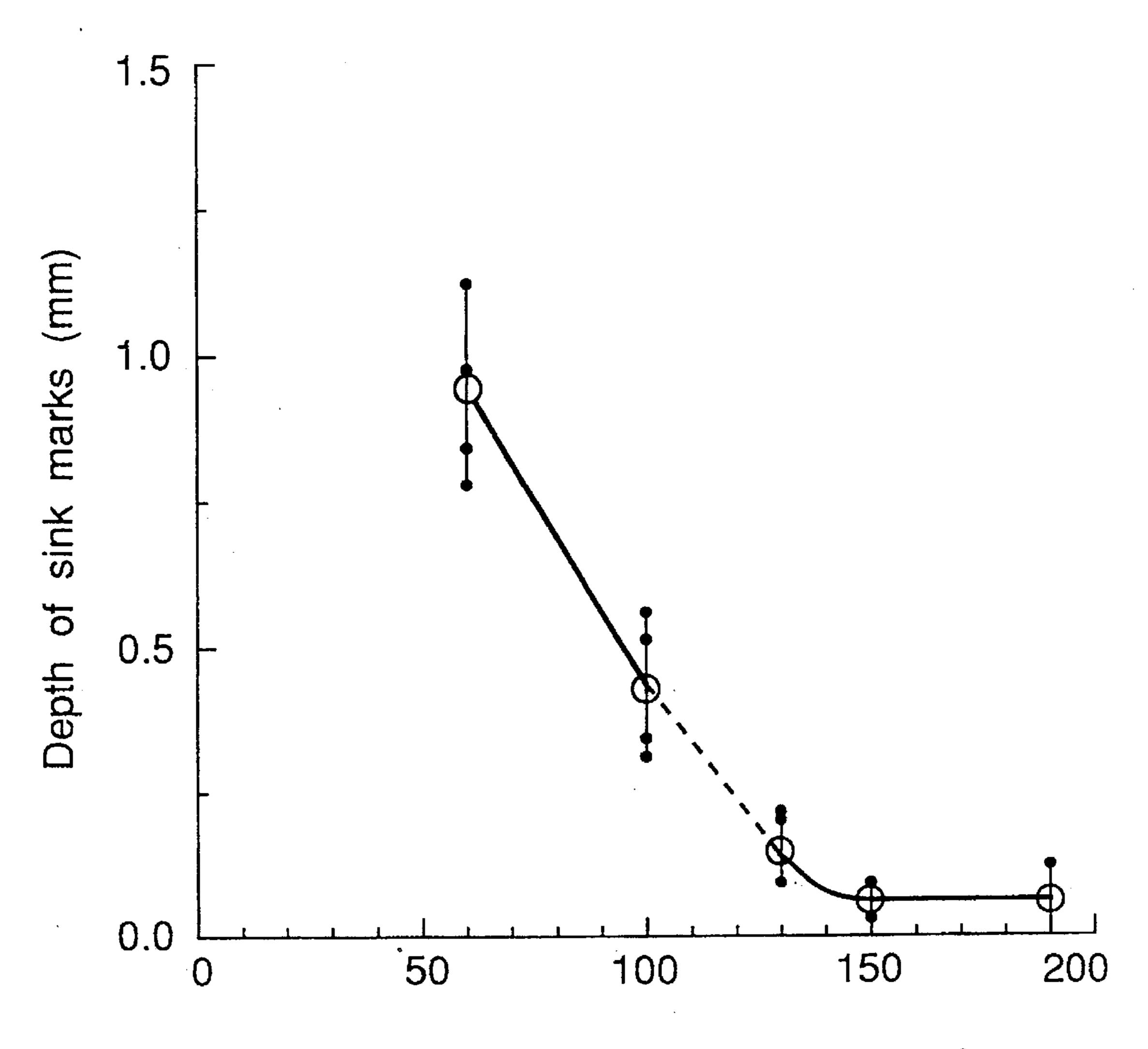
Wall surface temperature of mold (°C)
