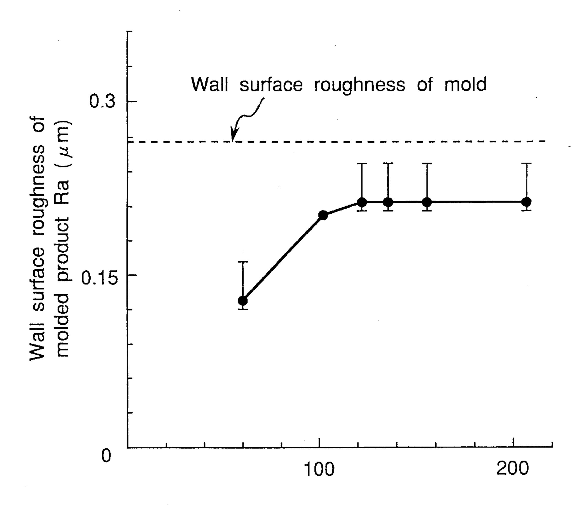
Wall surface temperature of mold (°C)
