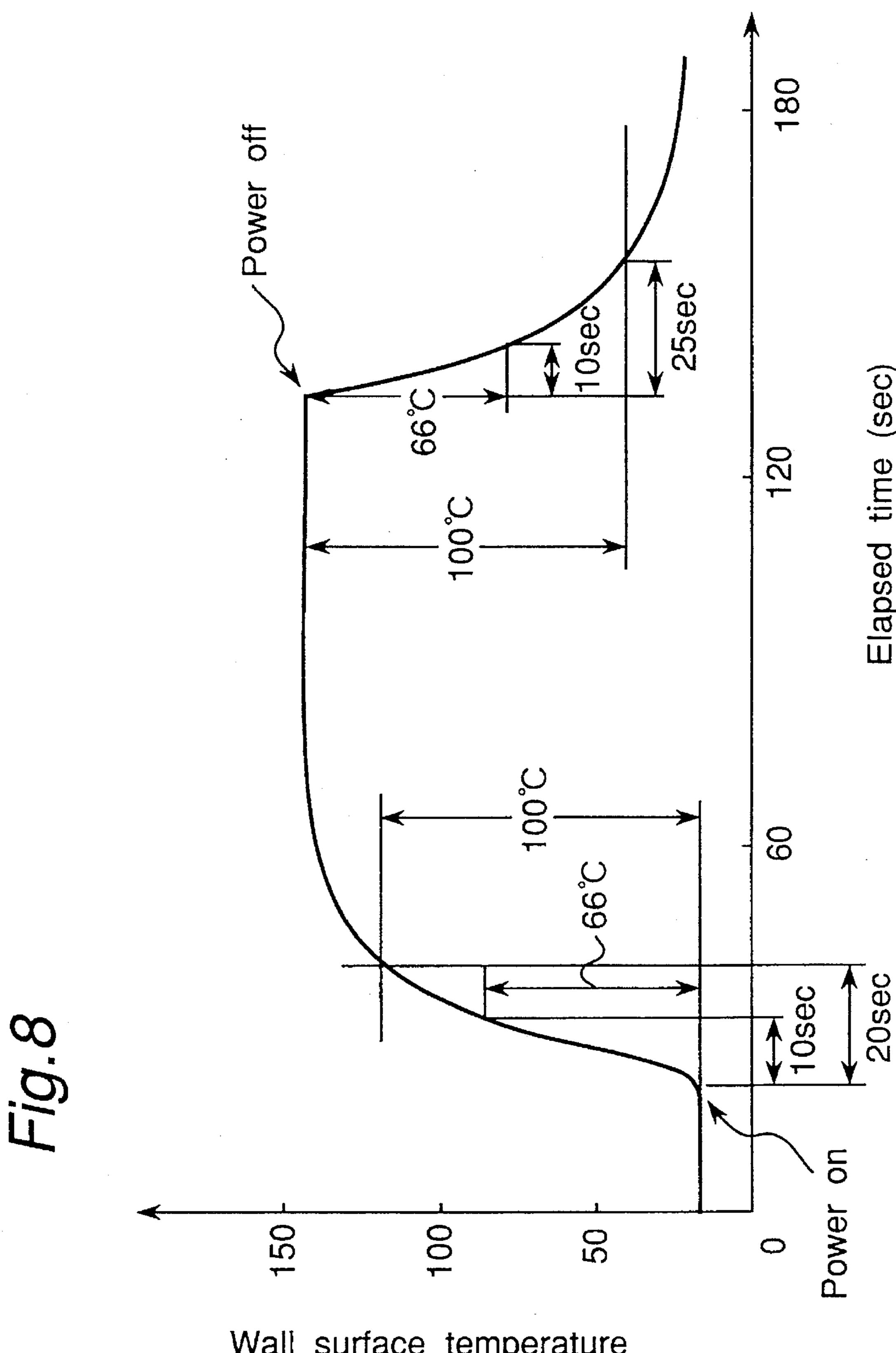
Wall surface temperature of mold (°C)
