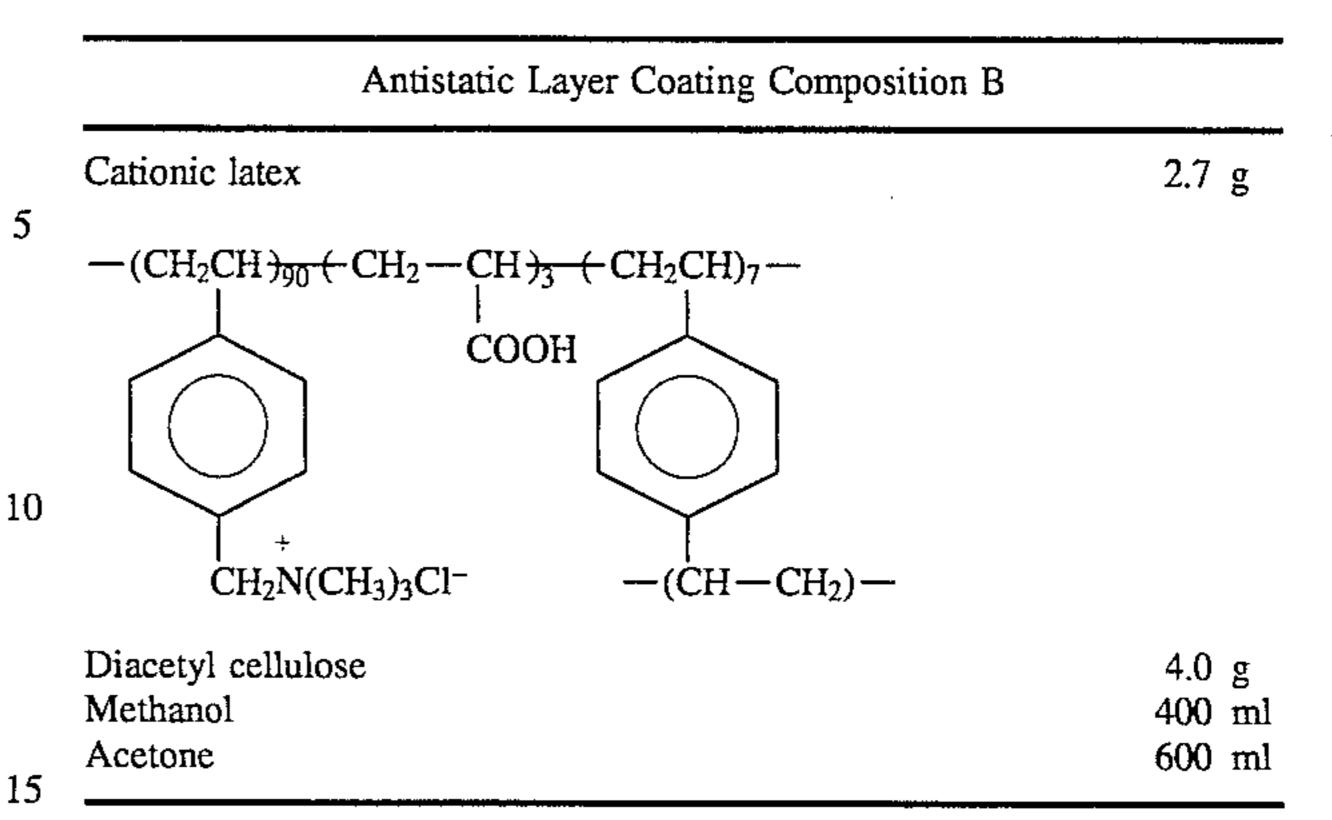
Onto the foregoing antistatic layer was coated the following slip layer coating composition B in an amount of 20 ml/m<sup>2</sup>. The material was then dried at a temperature of 100° C. for 3 minutes to form a slip layer.
