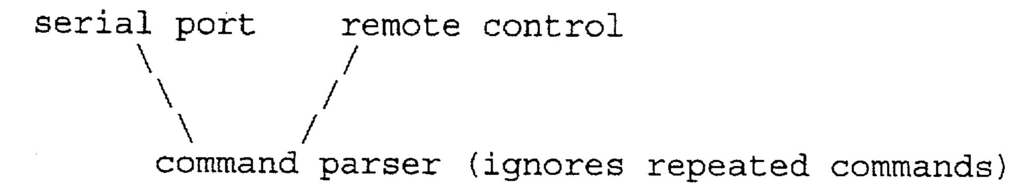
If a command is received through the serial port, it should bypass the IR RC pre-processor and accept repeated commands.
