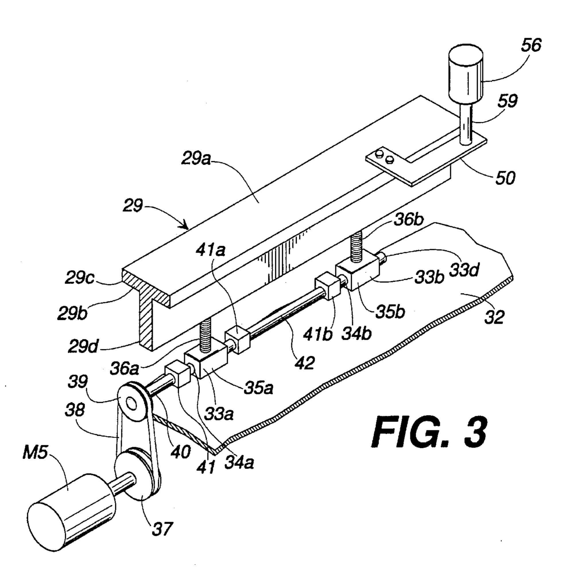
TUFTING MACHINE WITH PRECISION REMOTELY ADJUSTABLE BEDRAIL ASSEMBLY AND PROCESS OF CONTROLLING THE PILE HEIGHTS OF TUFTS TO BE PRODUCED ON A TUFTING MACHINE
