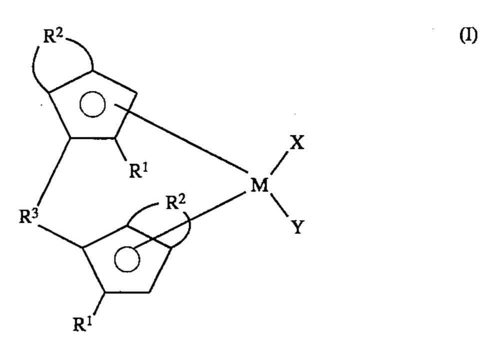
wherein:M represents a transition metal selected from the group consisting of titanium, zirconium and hafnium;
