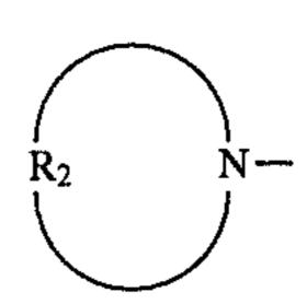
where each R<sub>1</sub> is independently selected from the group consisting of alkyls, cycloalkyls and aralkyls having from 1 to about 12 carbon atoms, and R<sub>2</sub> is a divalent alkylene, bicycloalkane, substituted alkylene, oxy- or N-alkylamino-alkylene group having from about 3 to about 16 methylene groups.
