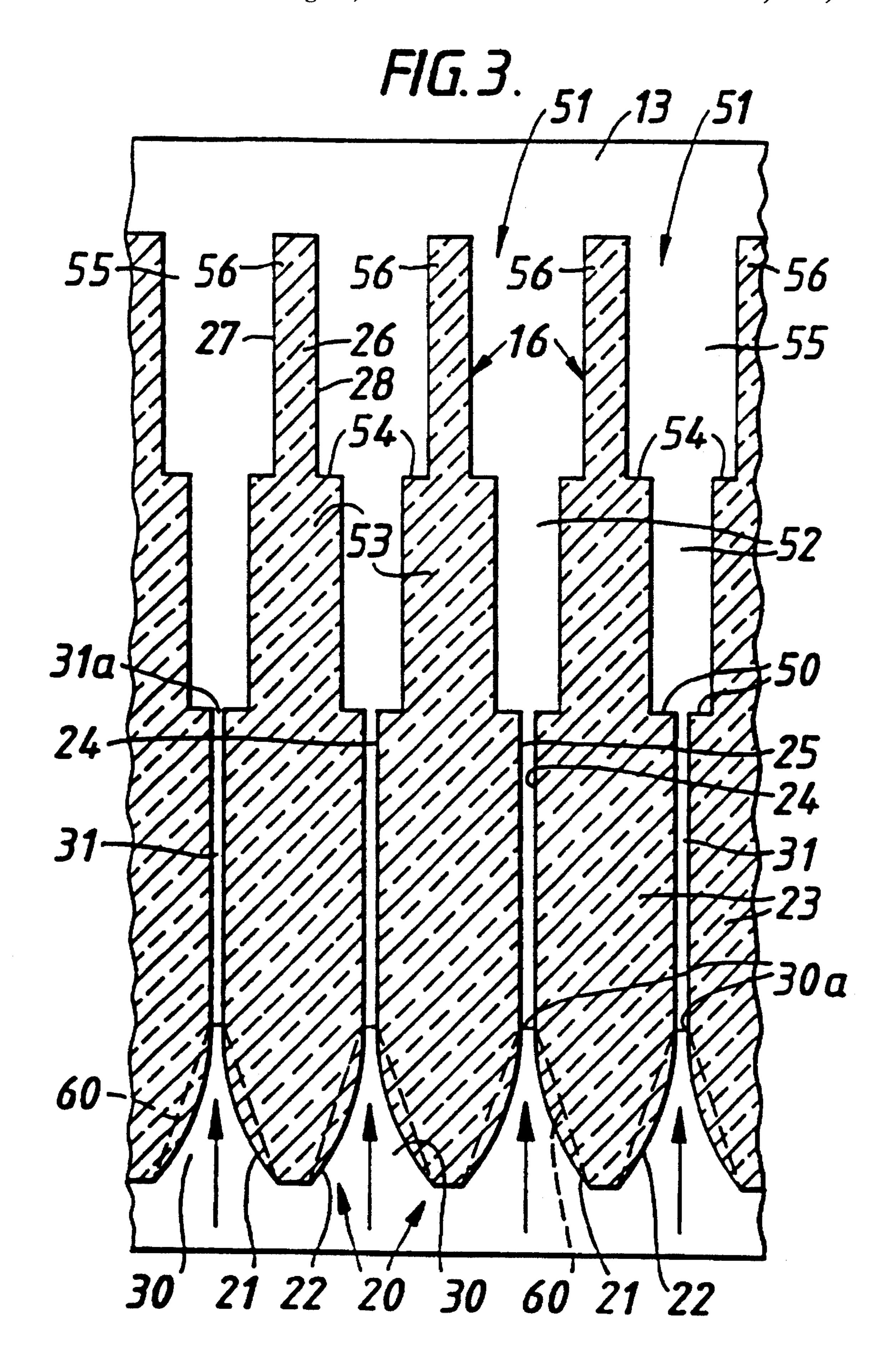
The present invention relates to a fuel-fired burner, and particularly a gas-fired burner, which preferably is of the fully premixed type i.e. one in which the fuel gas is mixed with all the combustion air in a mixing chamber before the gas is combusted.
