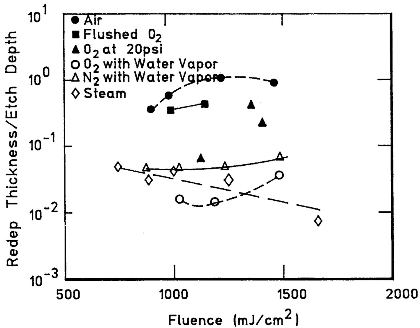
(Amount of Re-deposition at different etching conditions)
