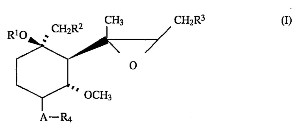
R<sup>2</sup> in the above formula (I) represents a halogen such as fluorine, chlorine, bromine or iodine. When R<sup>1</sup> and R<sup>2</sup> are combined to represent a chemical bond, they form an epoxy ring.
