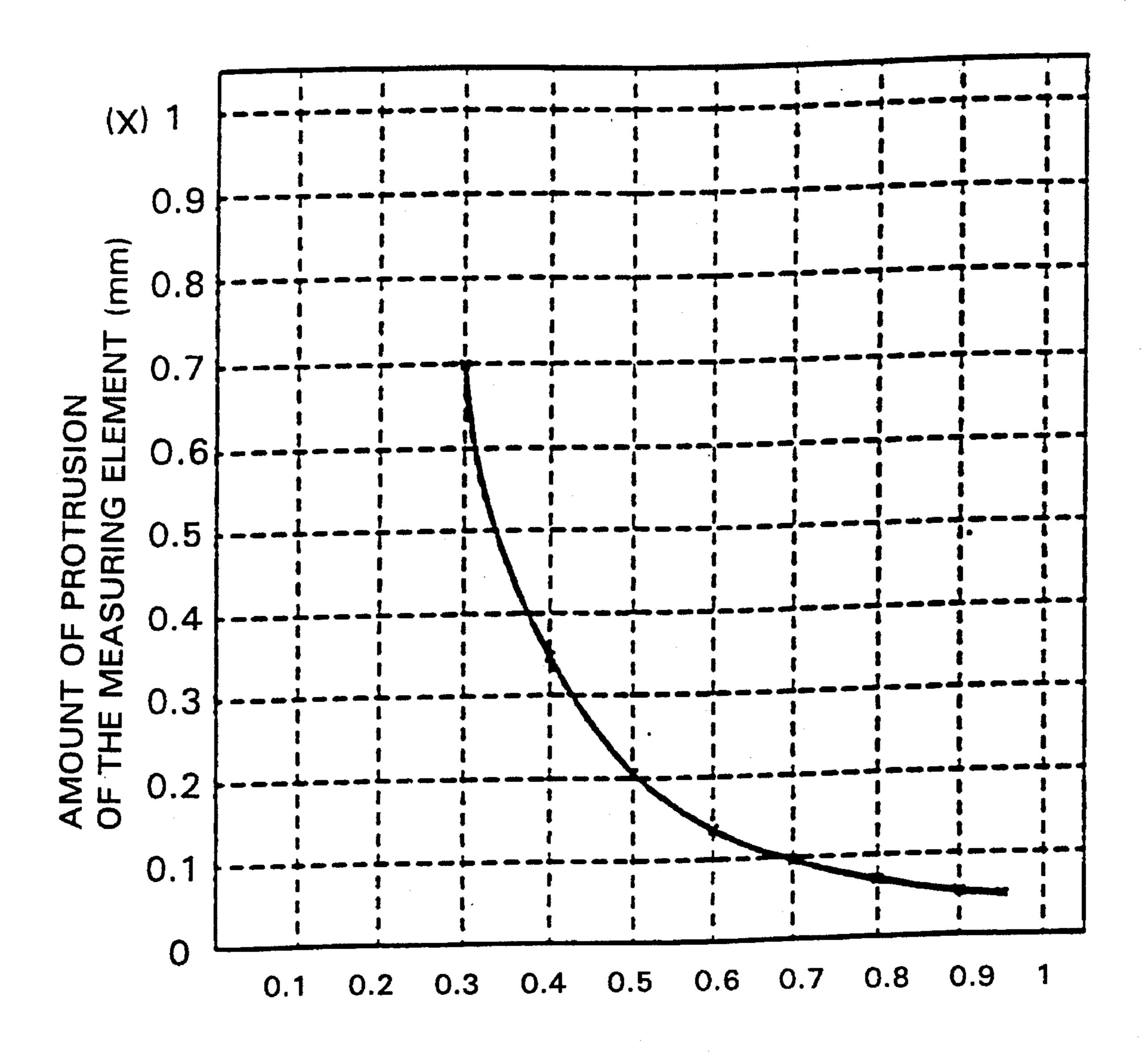
AMOUNT OF CHANGE IN THE SPINDLE (READING OF THE DIAL GAUGE)
