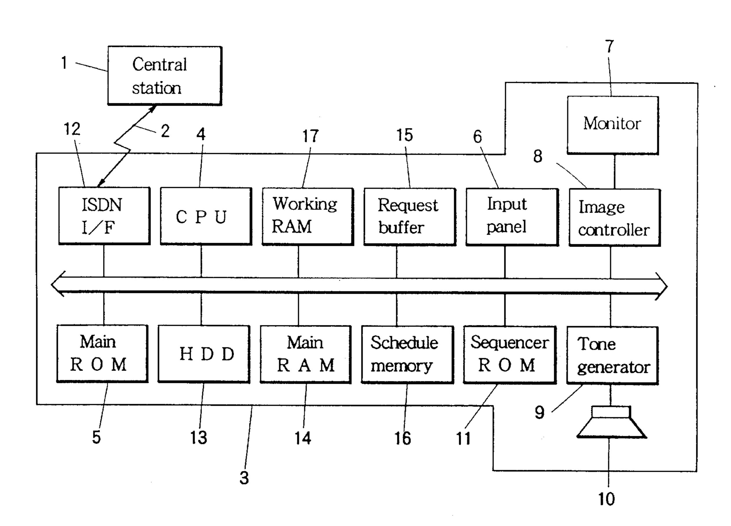
generator Image Tone Sequencer 6  $\infty$ Input panel 9 Request Schedule memory buffer 15 Working Main A RAM Д 4 Central station 8 Main 1
