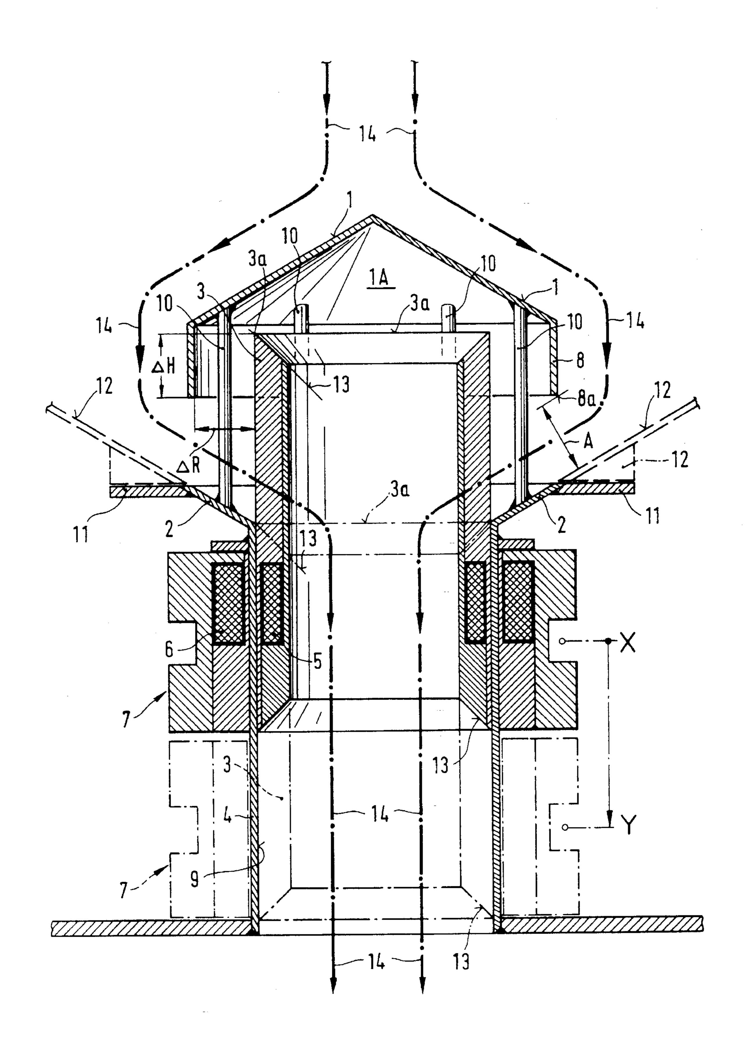
The invention relates to an annular dam slide valve for interrupting streams of bulk material flowing through the force of gravity.
