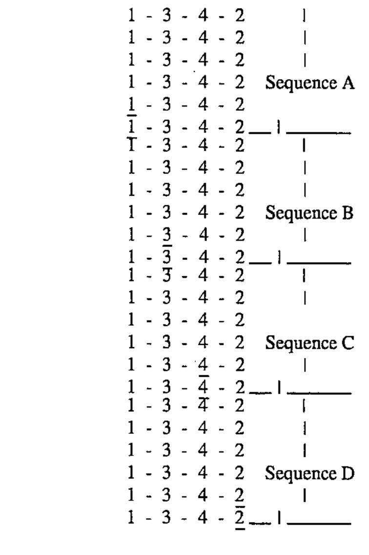
As indicated by the underlined cylinder number, cylinder 1 receives an interrupted fuel supply for two consecutive injection cycles, during injection sequence A. The fuel supply is then interrupted for two consecutive injection cycles to cylinders 3, 4 and 2, with a number of intervening
