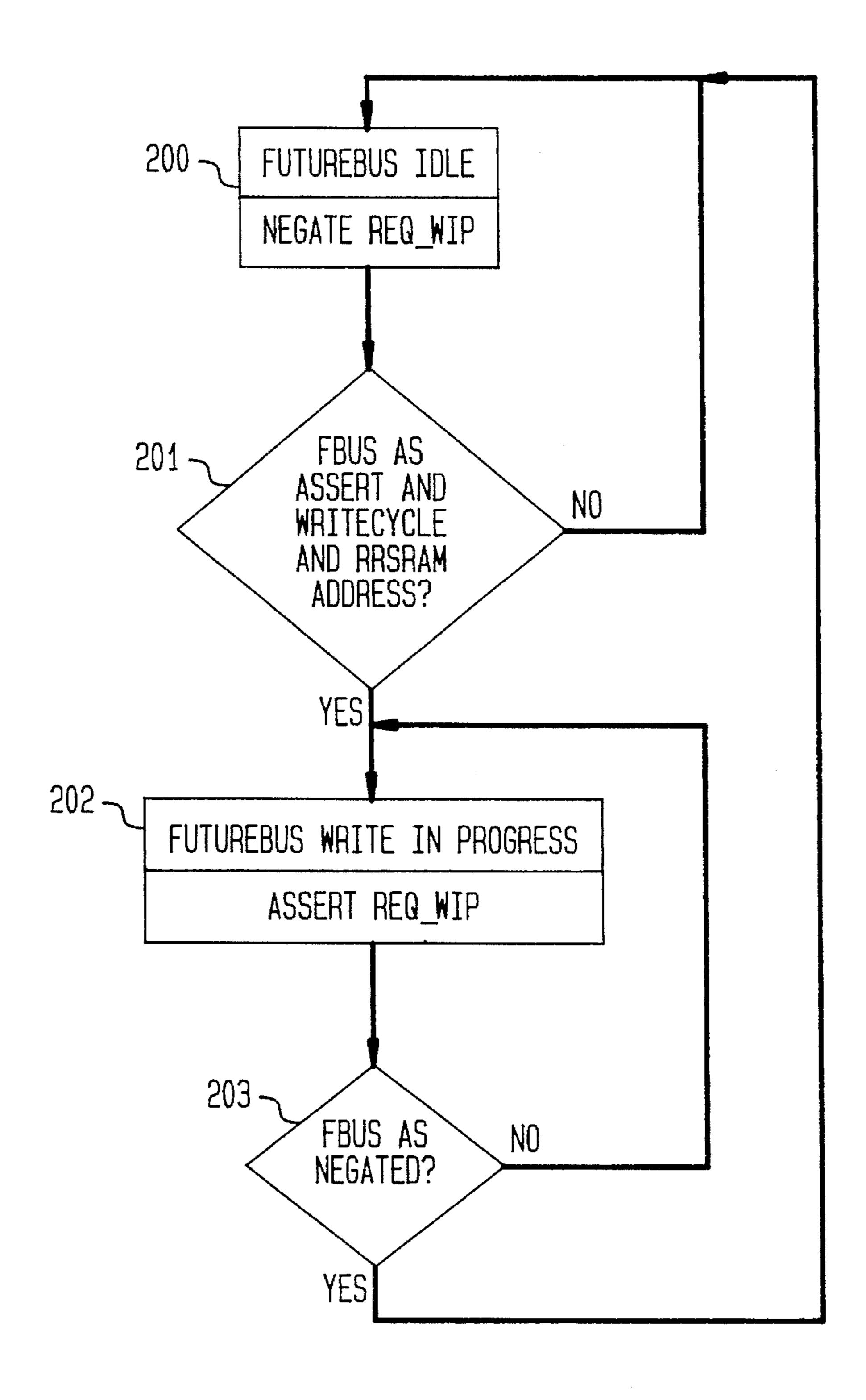
REQ\_WIP = REQUEST-WRITE-IN-PROGRESS FBUS\_AS = FUTUREBUS ADDRESS STROBE LWO RING = ADDRESS IN RRSRAM OF (RING AND RING ENTRY)
