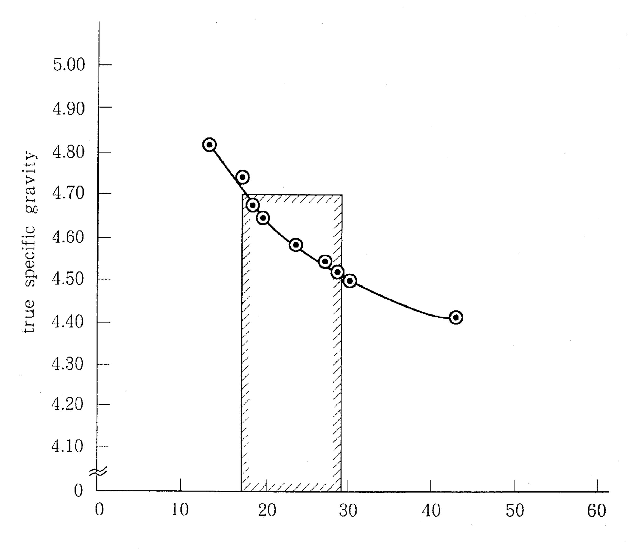
Li<sub>2</sub>O content (mol%) in ferrite particle core material
