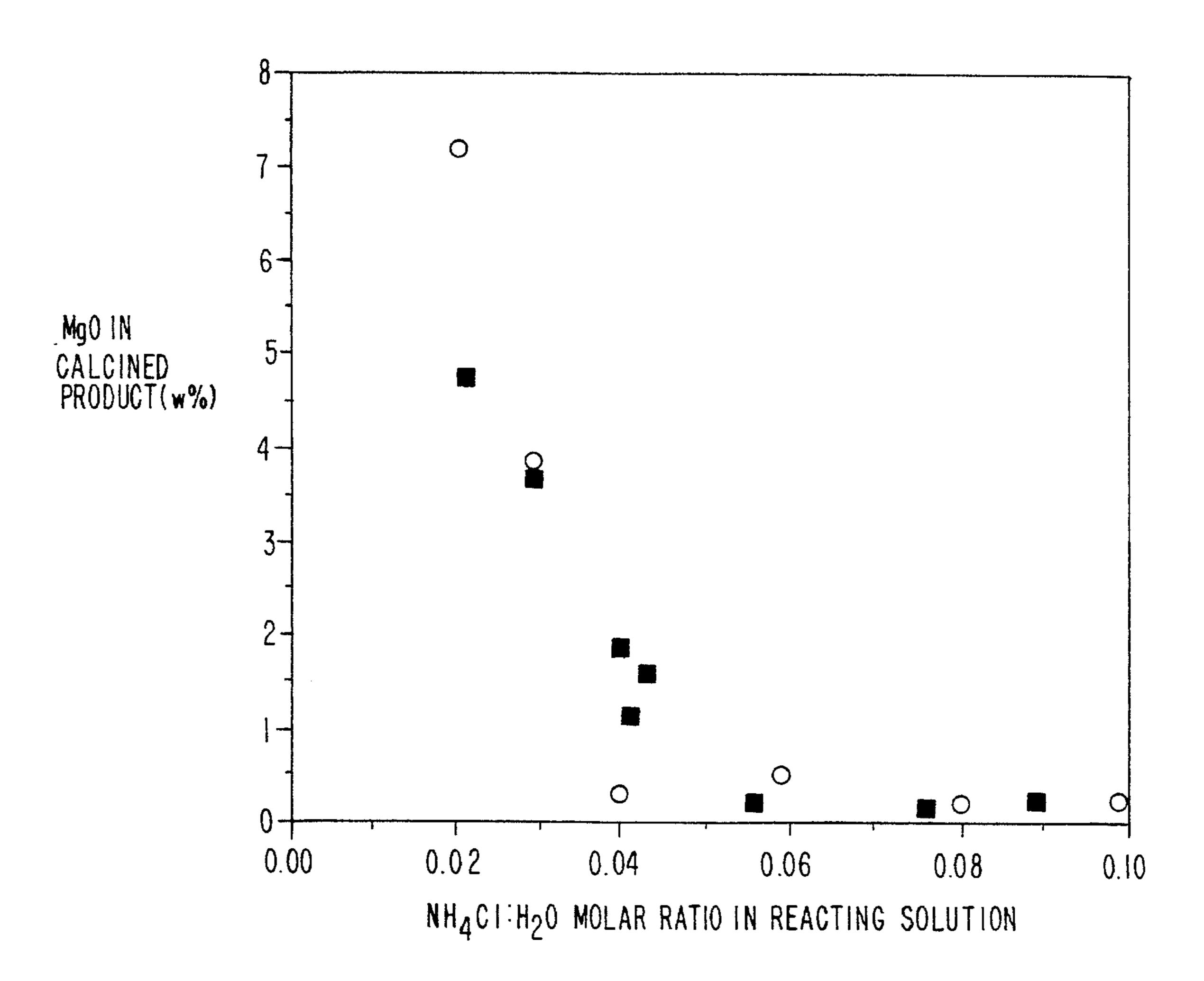
■Mg Cl<sub>2</sub> 2H<sub>2</sub>0 IN CH<sub>3</sub>0H FEED ○Mg Cl<sub>2</sub> 6H<sub>2</sub>0 IN CH<sub>3</sub>0H FEED
