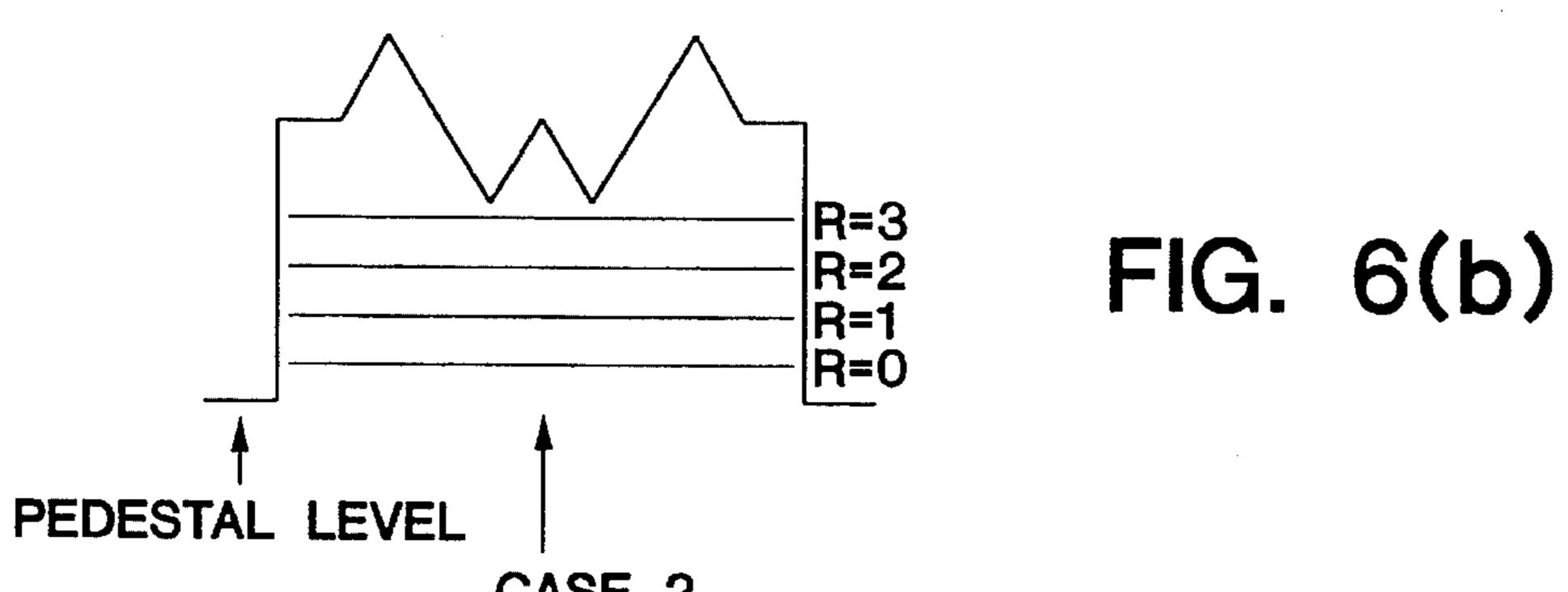
CASE 2 WHEN REFERENCE VALUE INITIAL SETTING  $R=0 \rightarrow R=1 \rightarrow R=2 \rightarrow R=3$ ; 4 TIMES WHEN REFERENCE VALUE INITIAL SETTING R=3; 1 TIME
