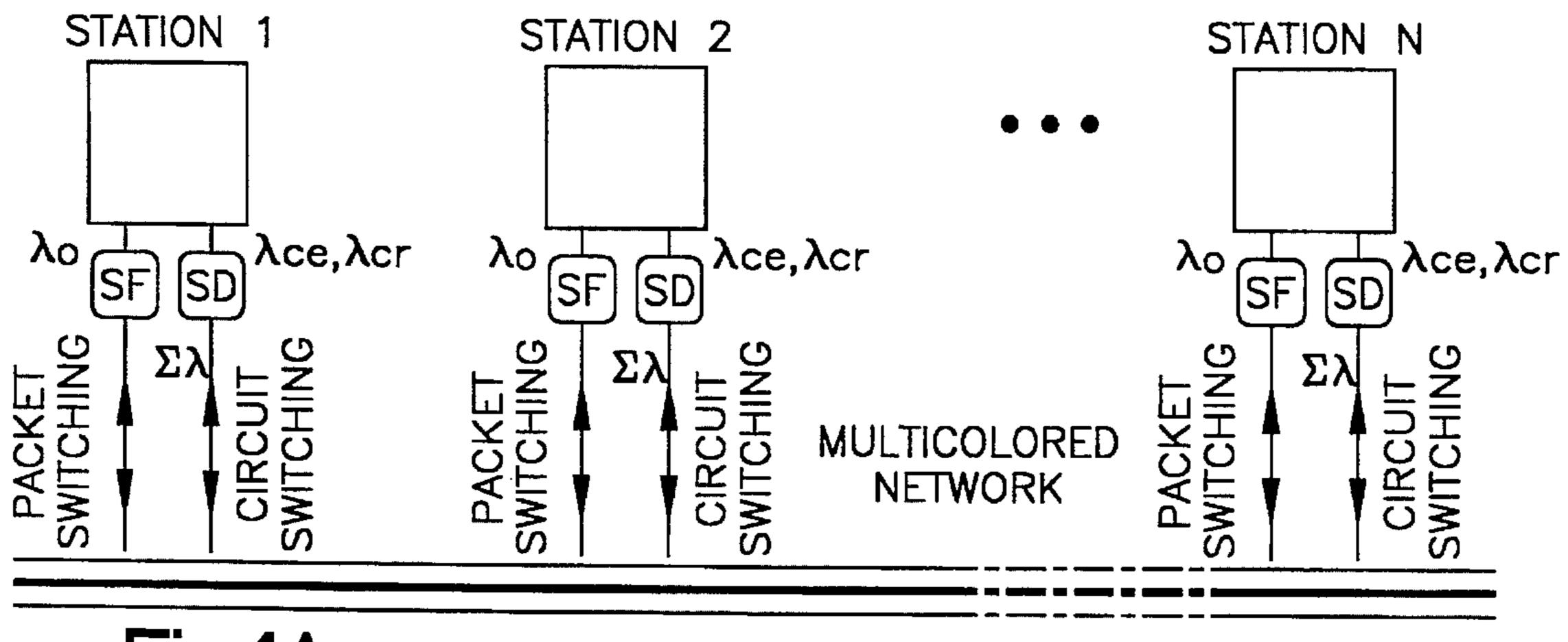
Fig.4A PACKET SWITCHING NETWORK
