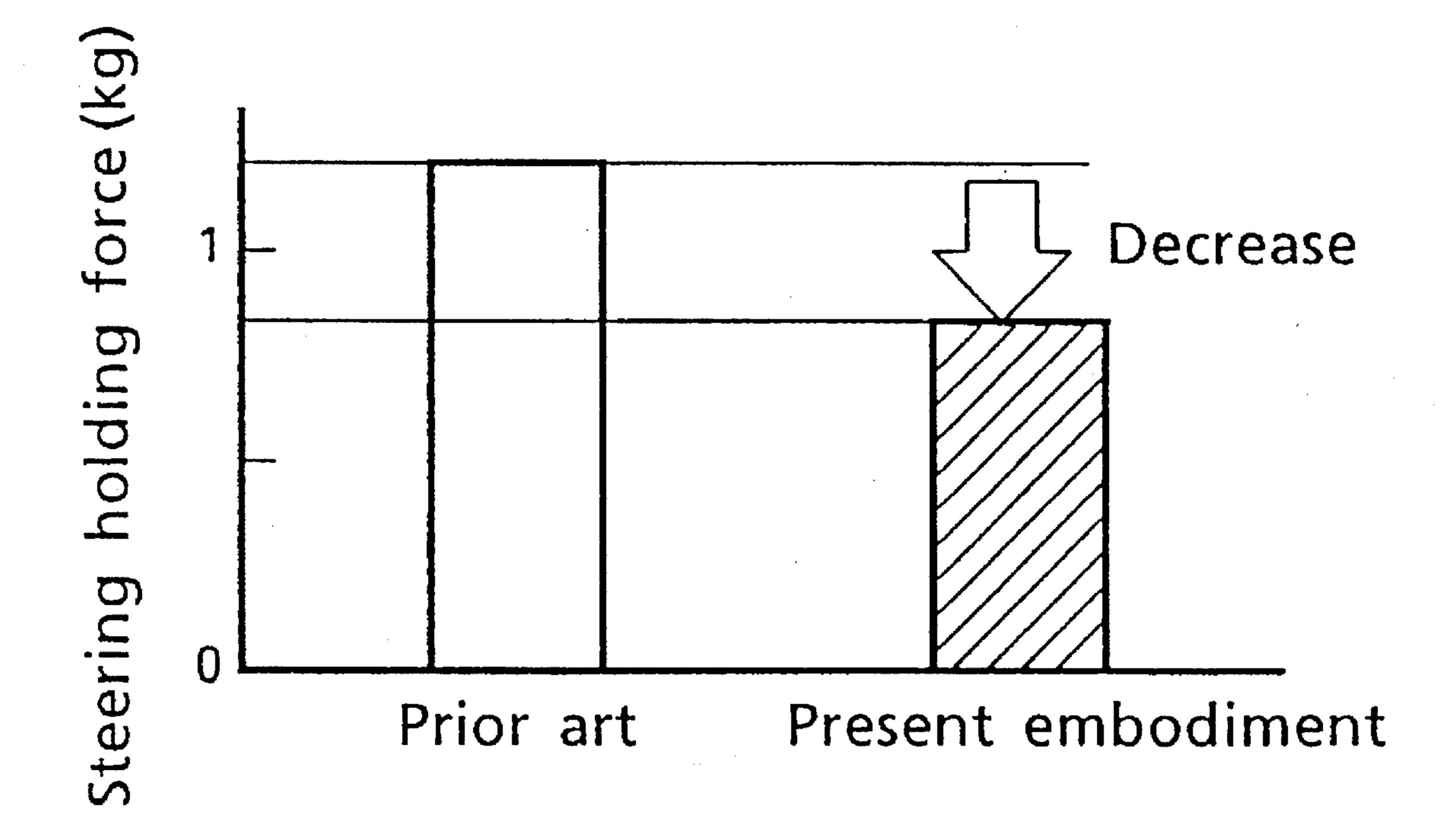
High speed running steer holding (V = 120 km/h, 600 mR turning)
