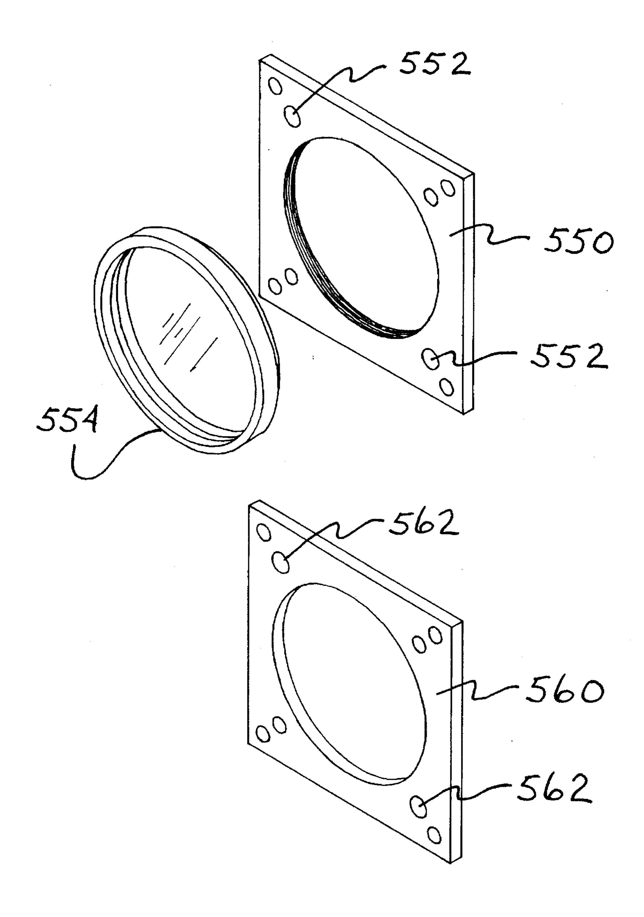
Figure 3 - Filter Holder and Spacer
