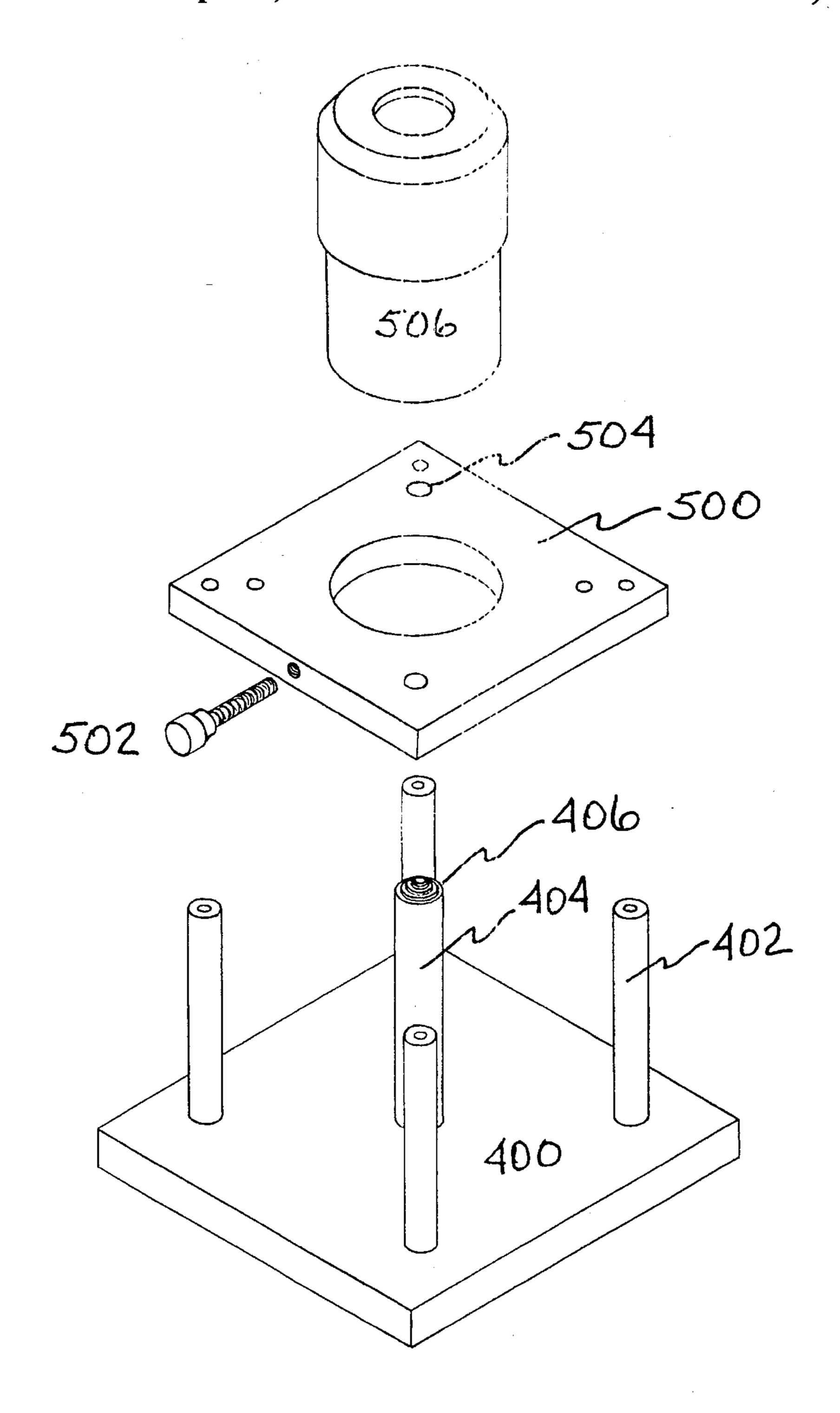
Figure 4 - Focus and Calibration Components
