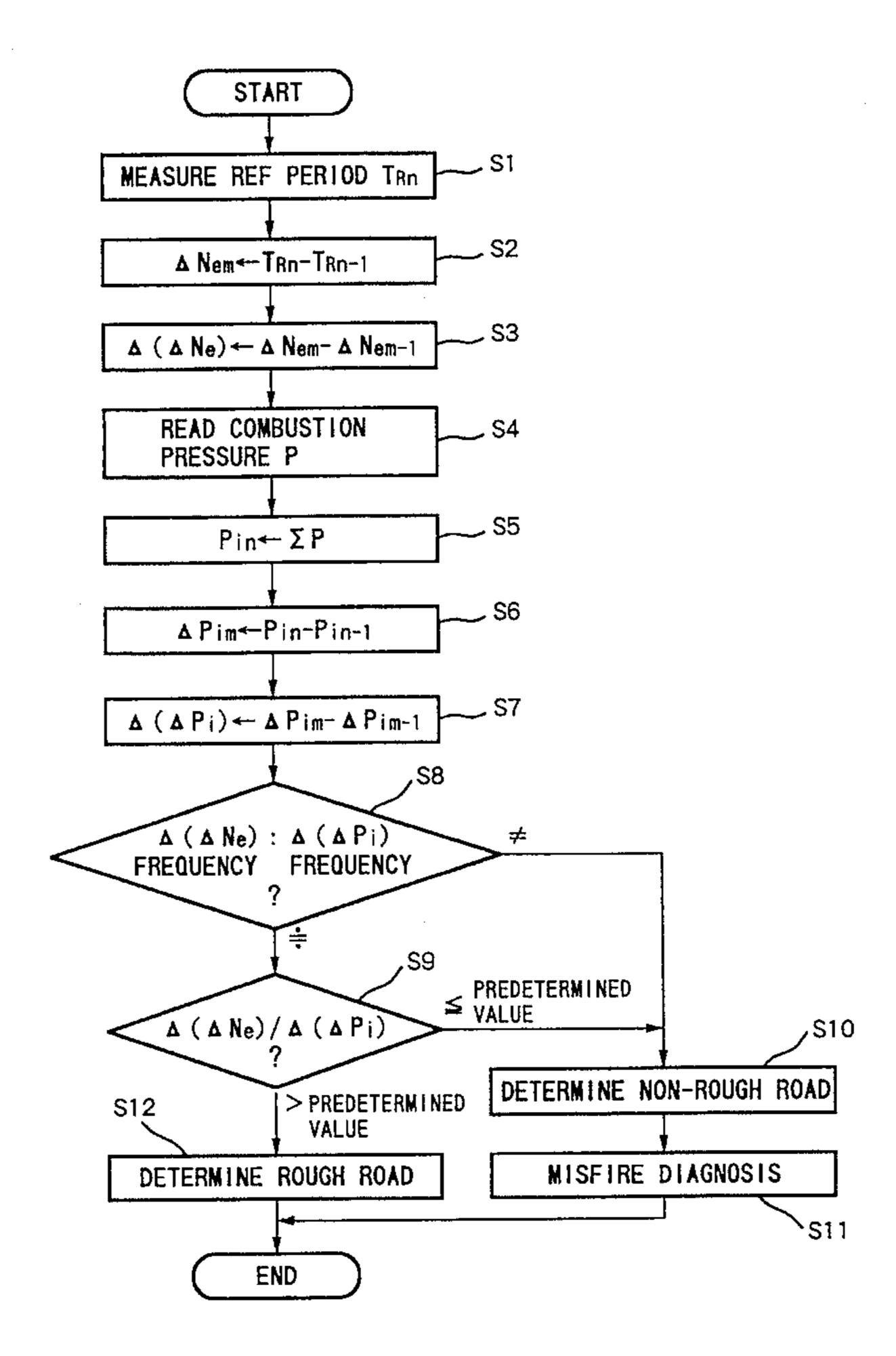
MISFIRE DETECTION DEVICE MISFIRE DETECTION INHIBIT DEVICE VEHICLE ENGINE MISFIRE DETECTION APPARATUS ROUGH ROAD TRAVEL DETECTION APPARTUS COMBUSTION PRESSURE DETECTION DEVICE ROTATIONAL SPEED DETECTION DEVICE
