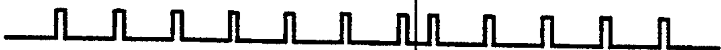
FIG. 5G OUTPUT SIGNAL OF OR CIRCUIT 66 SIGNAL (A) SHOWING CENTRAL POSITION OF GROOVE
