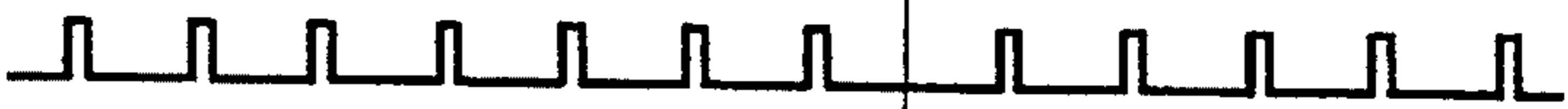
FIG. 5F OUTPUT SIGNAL OF OR CIRCUIT 65
