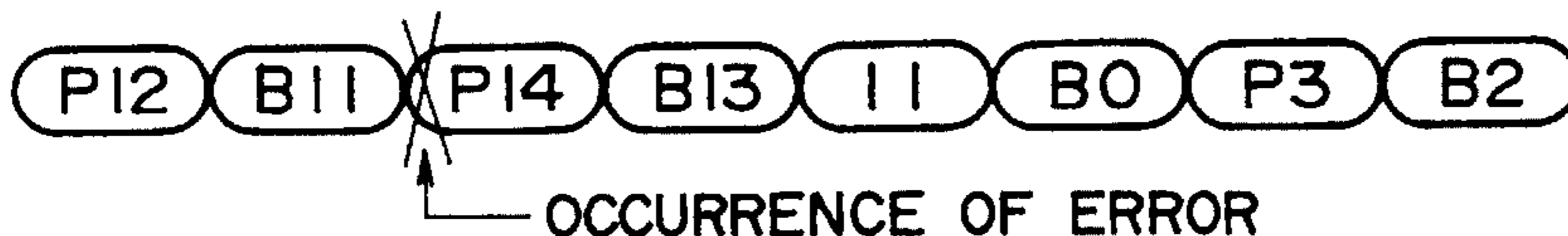
FIG. 3(c) VIDEO BIT STREAM (ERROR OCCURRENCE)
