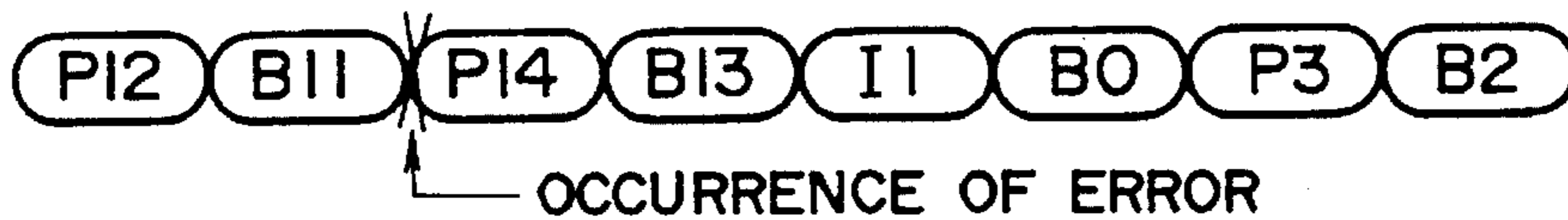
FIG. 9(c) VIDEO BIT STREAM (ERROR OCCURRENCE)
