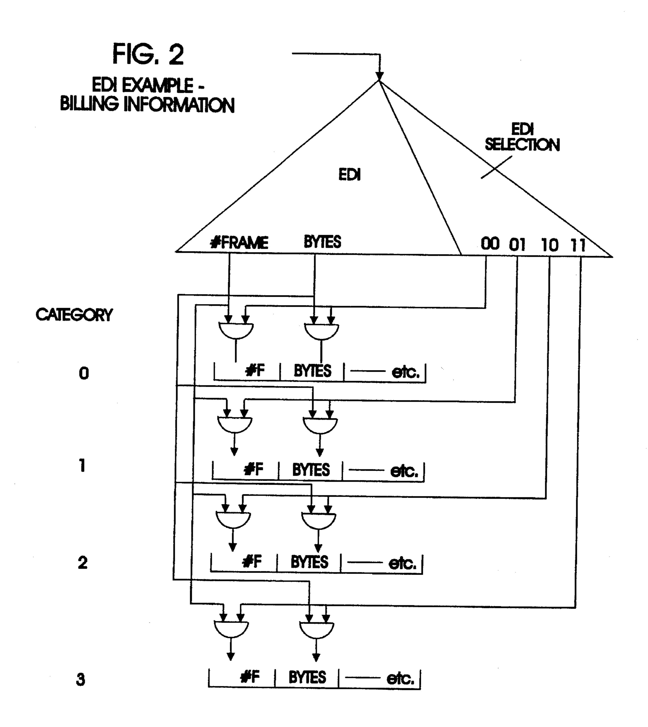
EXAMPLE: CATEGORIZING BILLING INFORMATION BY THE NUMBER OF FRAMES SENT (#F) AND THE NUMBER OF BYTES SENT (BYTES) BY DEVICES IN A FOUR NODE NETWORK WHERE DEVICE ADDRESSES ARE MAPPED BY THE EDI EXTENSION TO CATEGORY LOCATIONS 0, 1, 2, AND 3 IN RAM.
