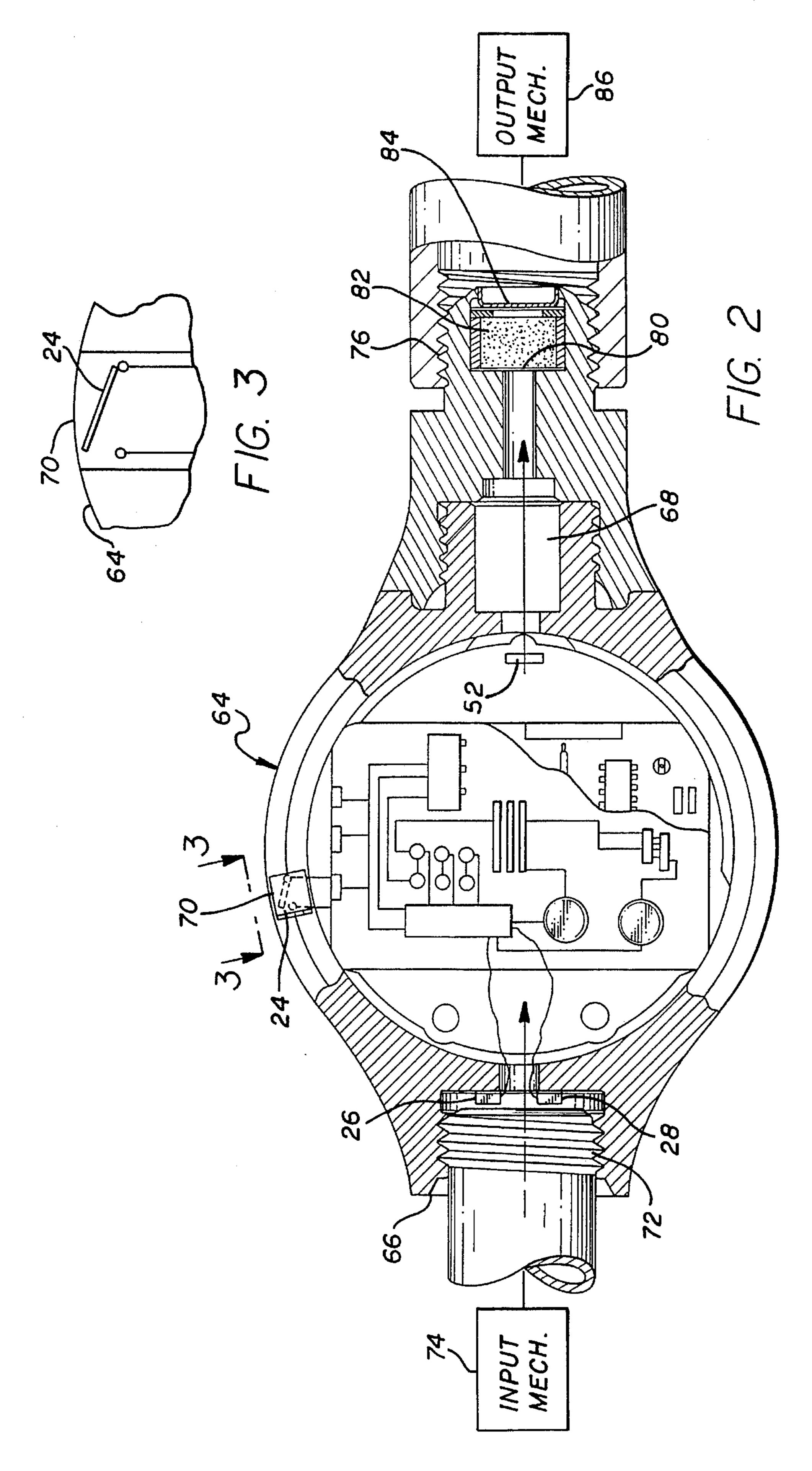
particularly, the invention relates to a delay ordnance system which includes any one of a plurality of input mechanisms, 5 any one of a plurality of output mechanisms and an electronic timing and firing system adapted to be coupled on a universal basis to individual ones of the input and output mechanisms.
