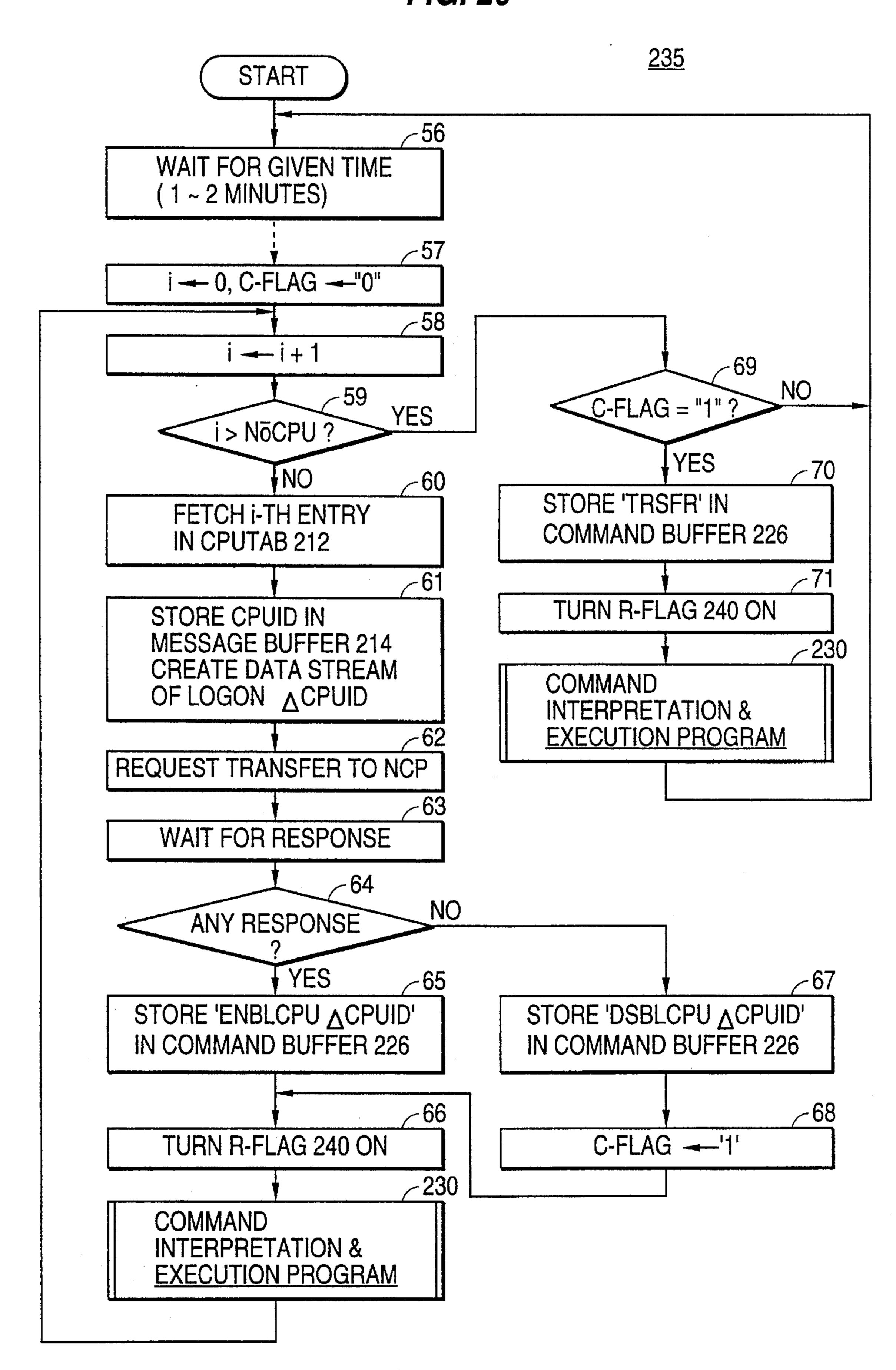
SYSTEM FOR DYNAMICALLY SWITCHING LOGICAL SESSIONS BETWEEN TERMINAL DEVICE AND A PROCESSOR WHICH STOPS ITS OPERATION TO ANOTHER WORKING PROCESSOR UNDER CONTROL OF COMMUNICATION CONTROL PROCESSOR
