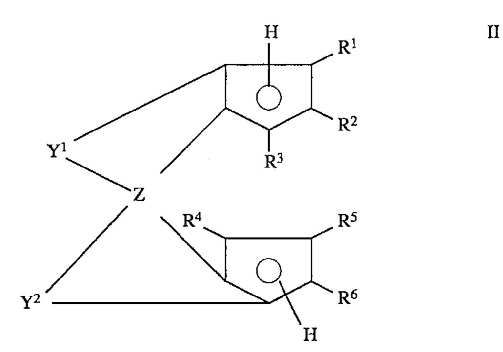
The cyclopentadienyl compounds II can be converted into the metallocene complexes I by reaction with metalating agents, such as alkali metal alkyls, alkaline earth metal alkyls, alkali metal hydrides or alkaline earth metal hydrides, preferably n-butyllithium, and subsequent addition of  $MX_4$ .
