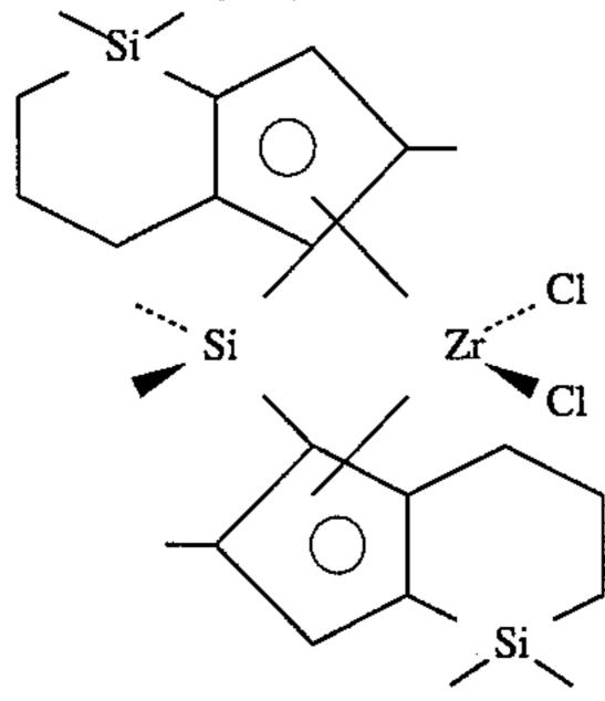
\*2: Dimethylsilylenebis(4,5,6,7-tetrahydroindenyl)zirconium dichloride
