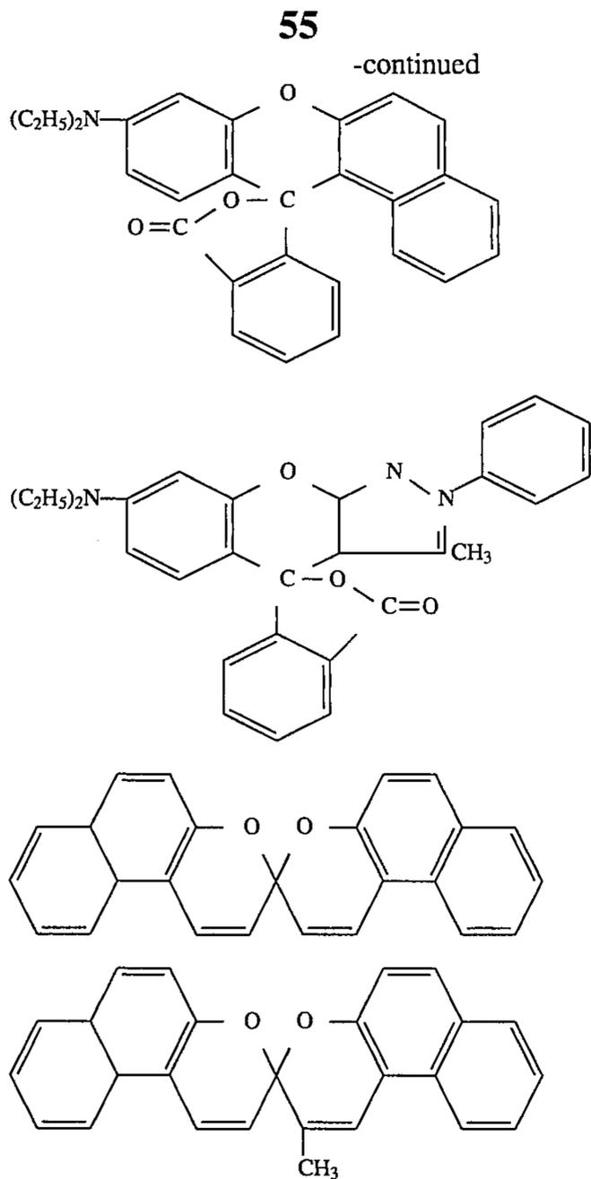
A memory effect imparting agent selected from among the above substances is added in the ratio of 0.001 to 1 part by weight, particularly 0.001 to 0.1 part by weight, to 1 part by weight of an organic photoconductive substance. If the amount of memory effect imparting agent added exceeds 1 part by weight, the amplifying function of the photoelectric sensor markedly lowers, which is unfavorable.
