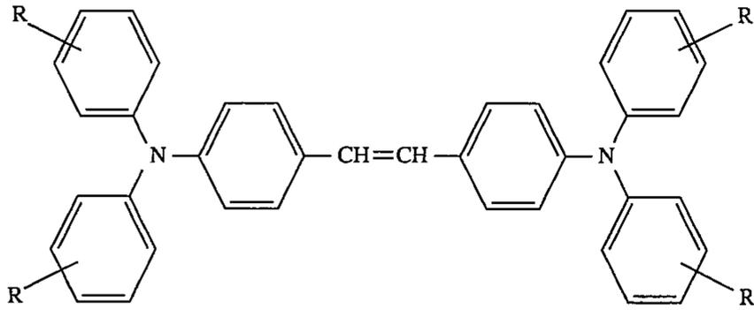
R represents methyl, methoxy, chlorine in ortho, meta, para positions.
