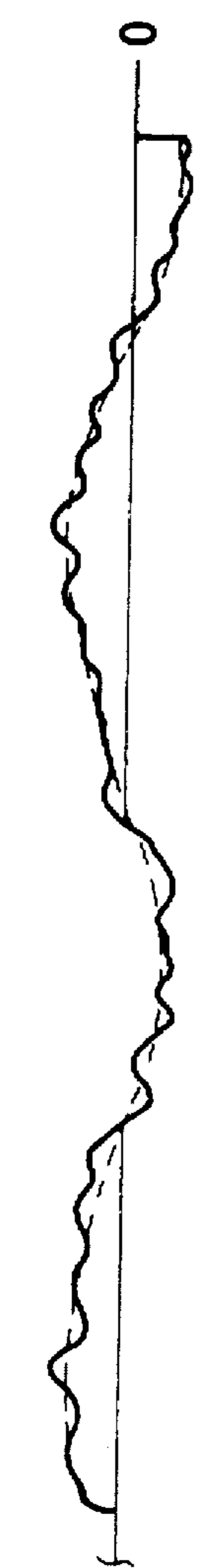
ACTUAL SAMPLING WAVEFORM (EXTRACTION OF D.C. OFFSET)
