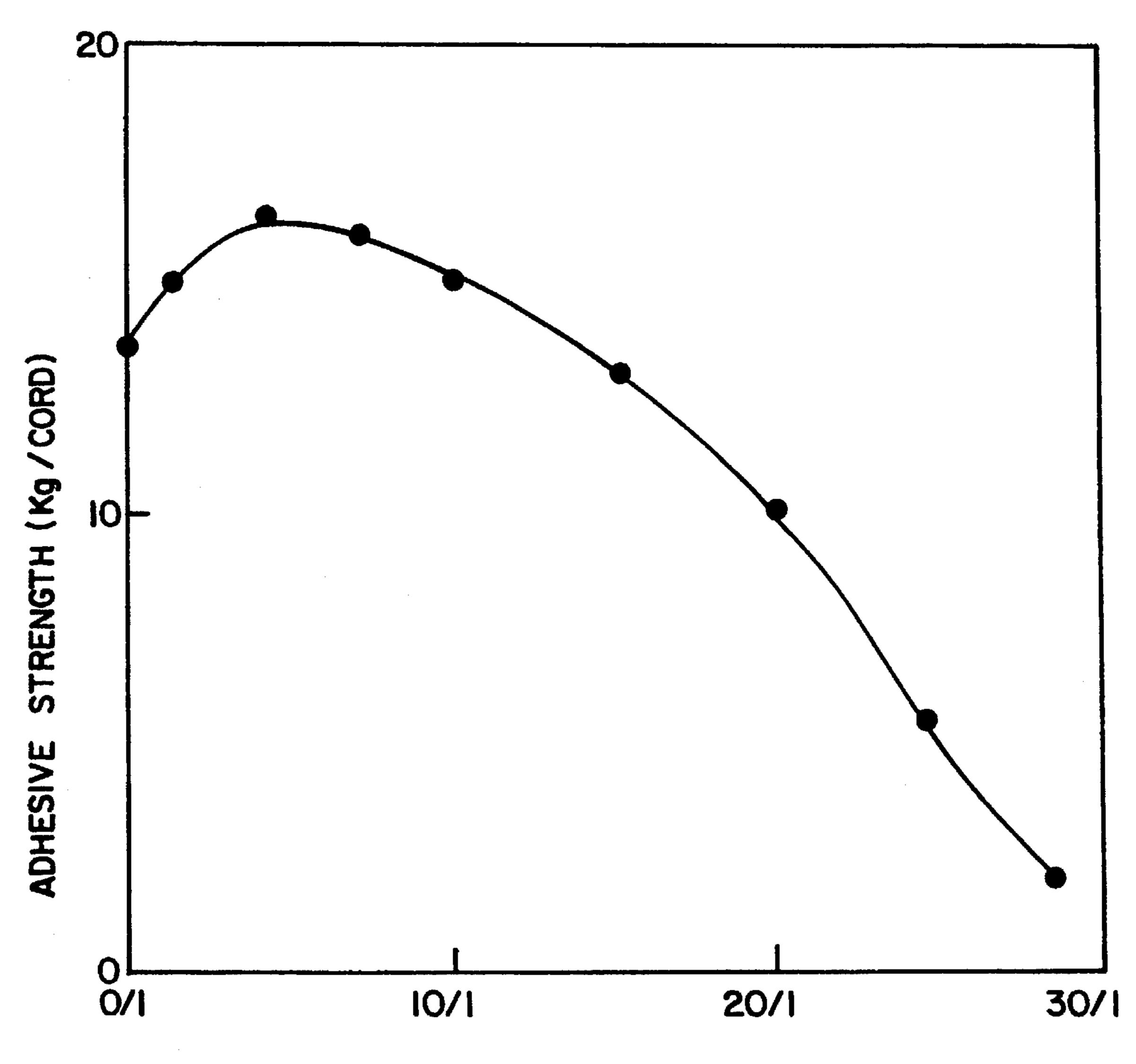
WEIGHT RATIO OF CHLORINATED NATURAL RUBBER / ADHESIVE RUBBER
