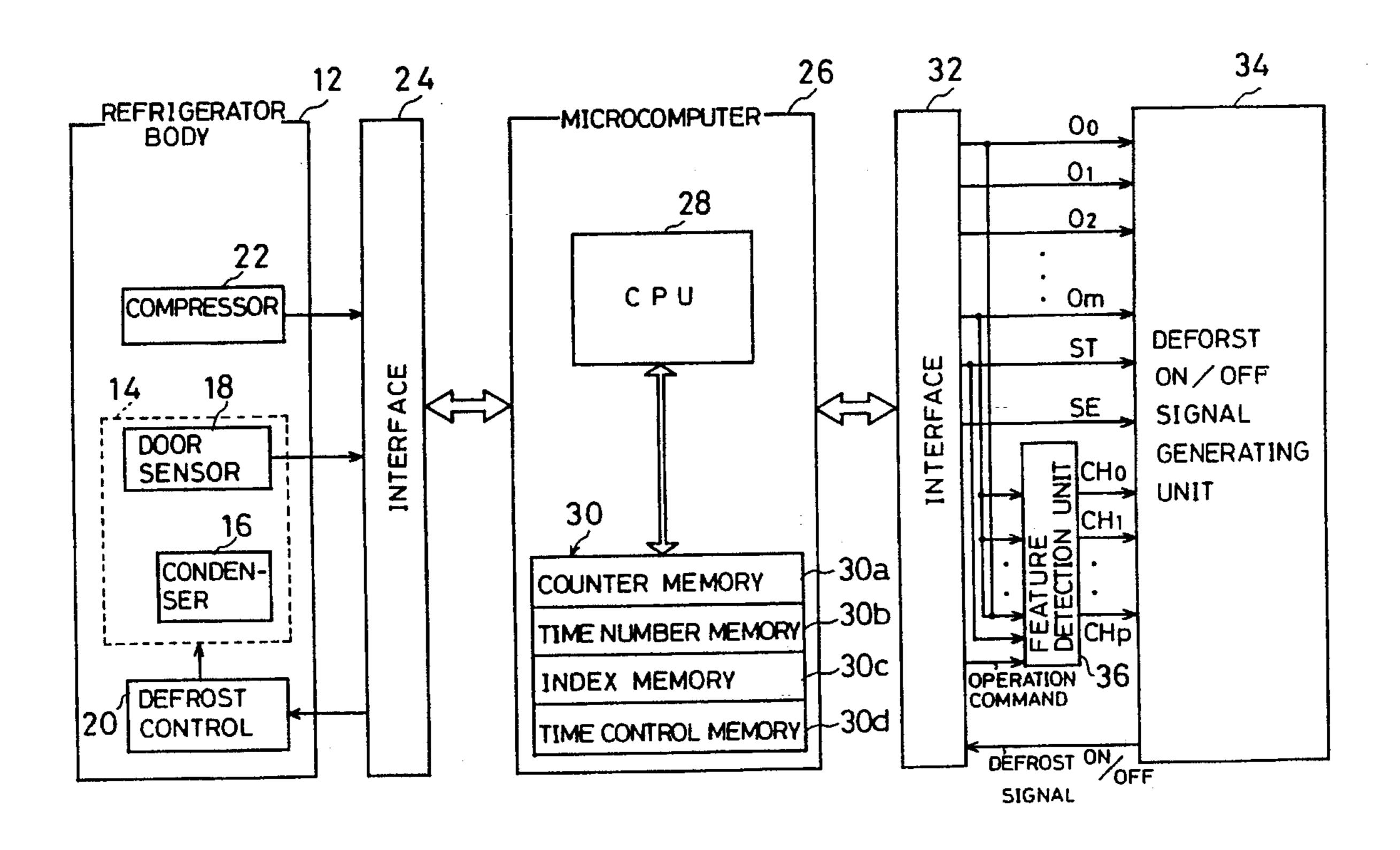
SE S DEFROST SIGNAL FEATURE 32 INTERFACE 30b 26 MEMDRY TIME NUMBER MEMORY MEMORY MEMORY 28 HROL. INDEX TIME 2 INTERFACE COMPRESSOR CONDEN CONTROL NSOR
