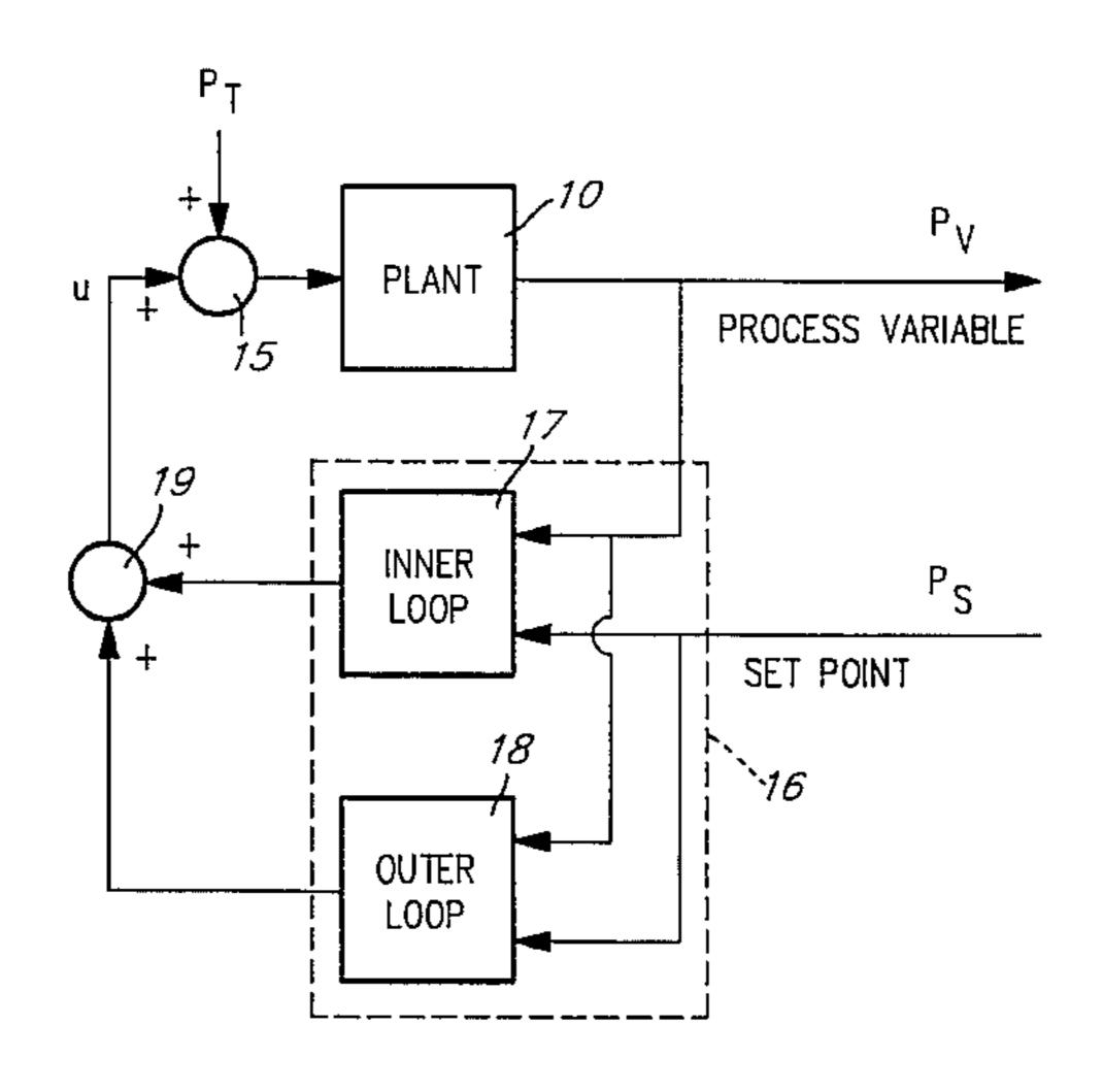
the sensitivity through the gains of the outer loop does not change the input/output characteristics of the controller that have been previously adjusted by means of the gains of the inner loop after having set the gains of the outer loop equal
