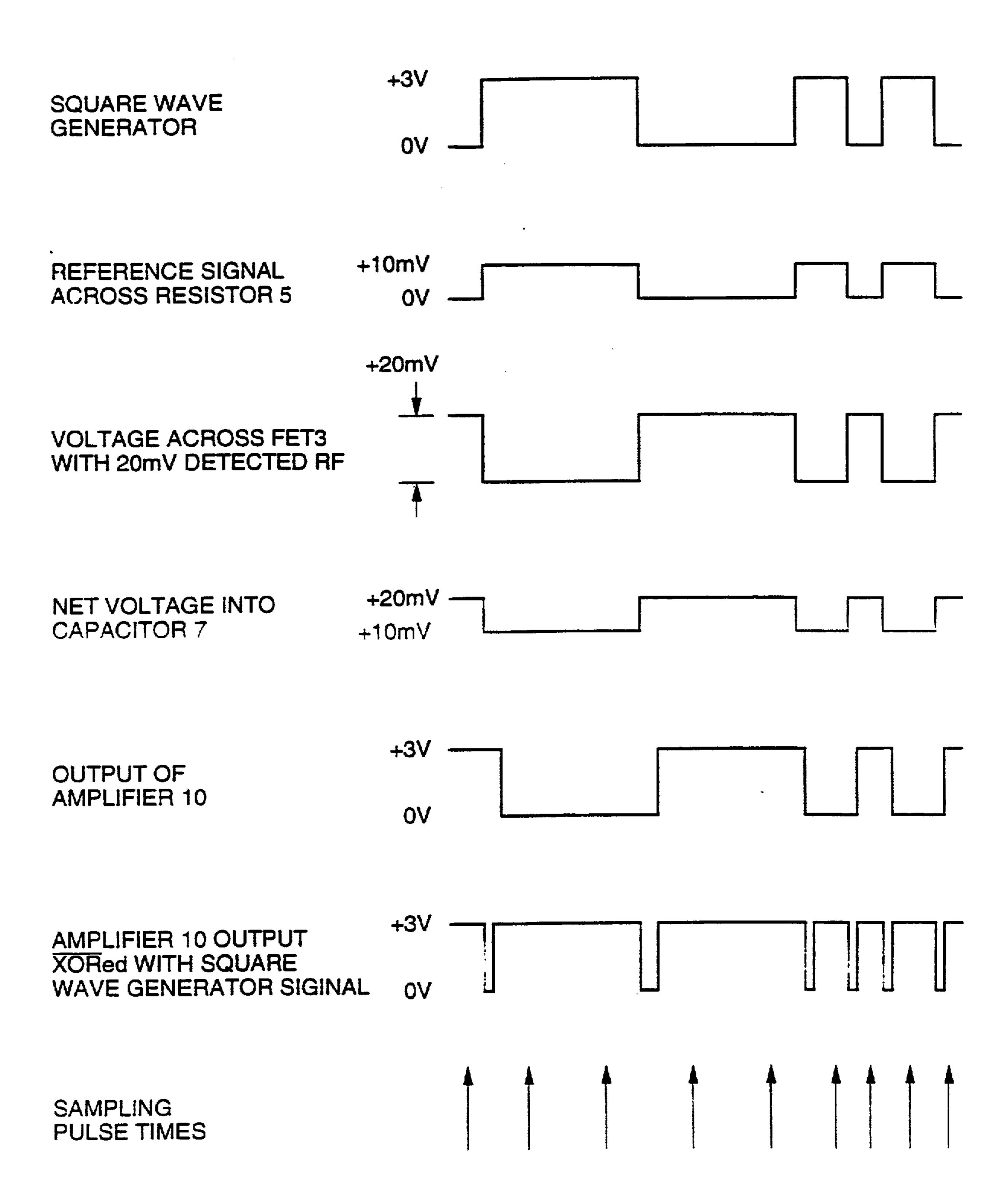
SIGNAL WAVE SHAPES WITH DETECTED RF OF 20mV, LARGER THAN THE 10mV REFERENCE SIGNAL.
