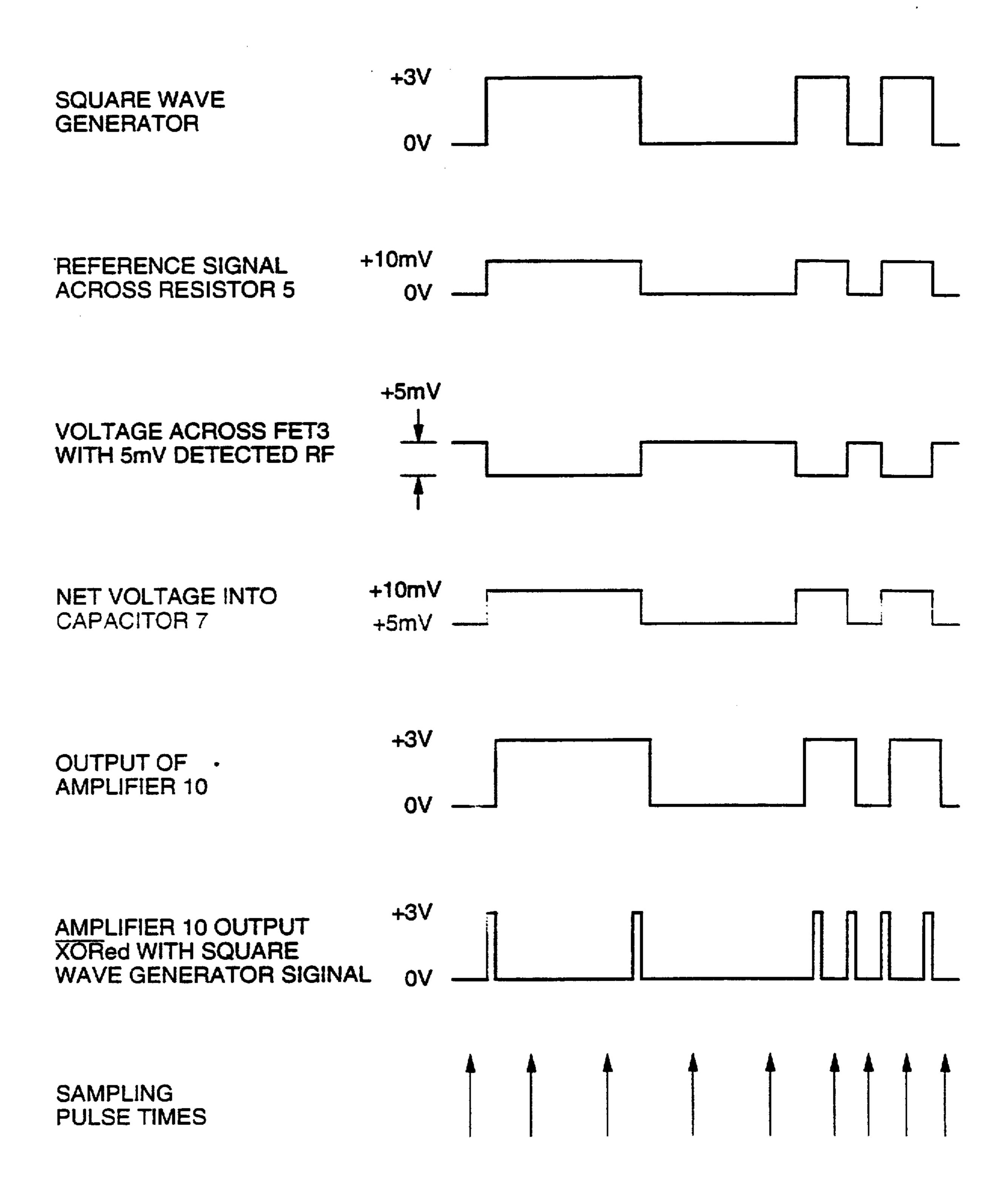
SIGNAL WAVE SHAPES WITH DETECTED RF OF 5mV, SMALLER THAN THE 10mV REFERENCE SIGNAL.
