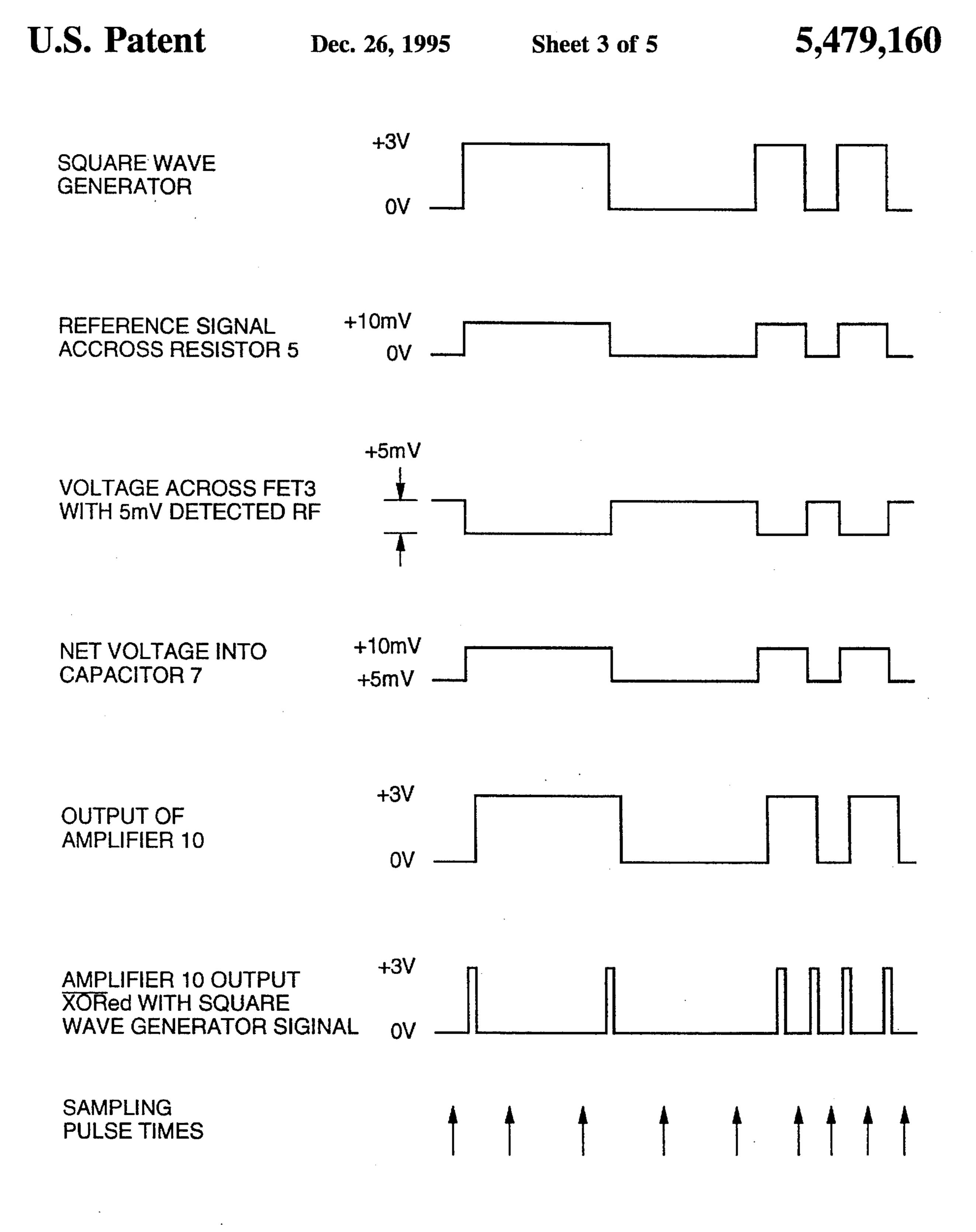
SIGNAL WAVE SHAPES WITH DETECTED RF OF 5mV, SMALLER THAN THE 10mV REFERENCE SIGNAL.
