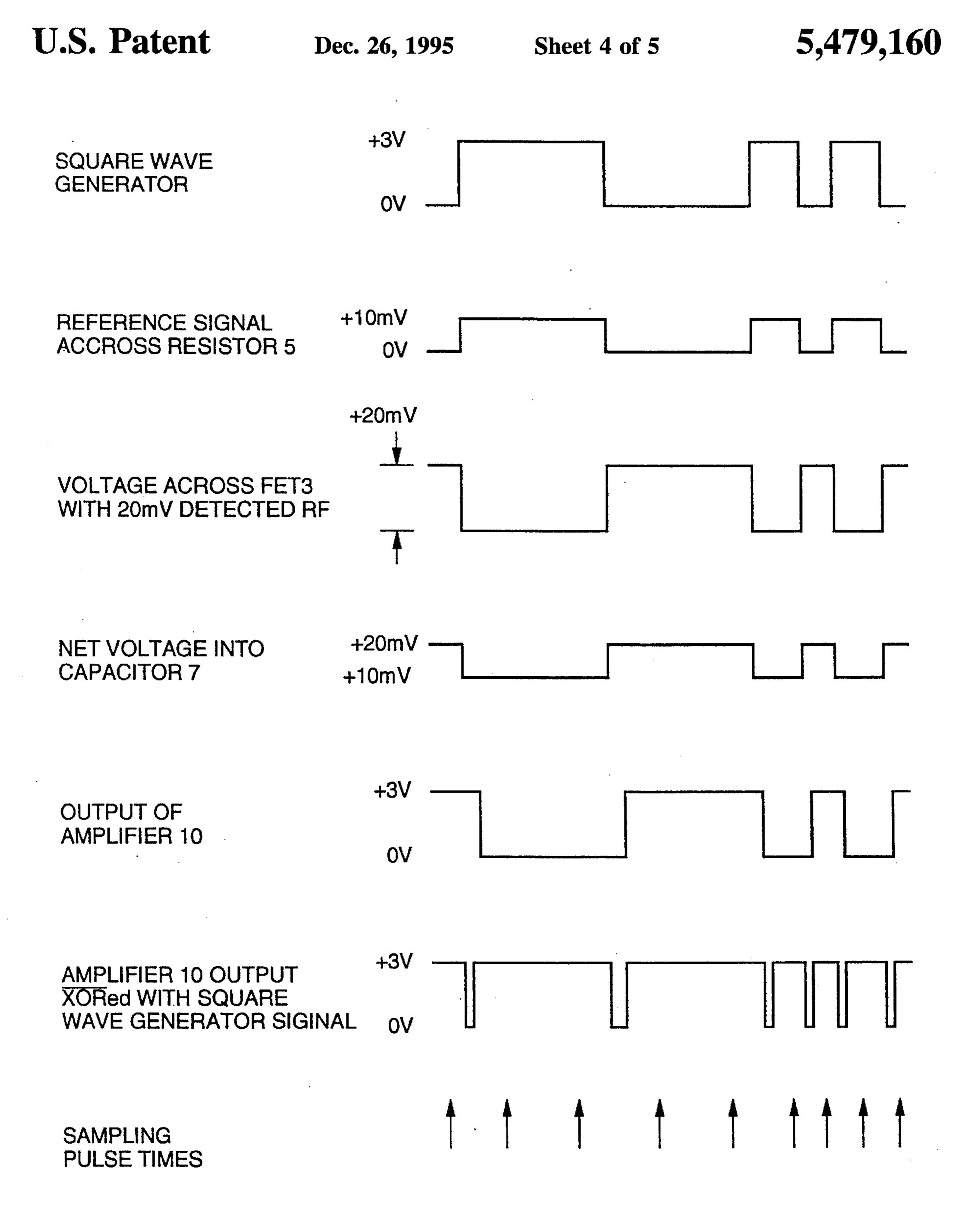
SIGNAL WAVE SHAPES WITH DETECTED RF OF 20mV, LARGER THAN THE 10mV REFERENCE SIGNAL.
