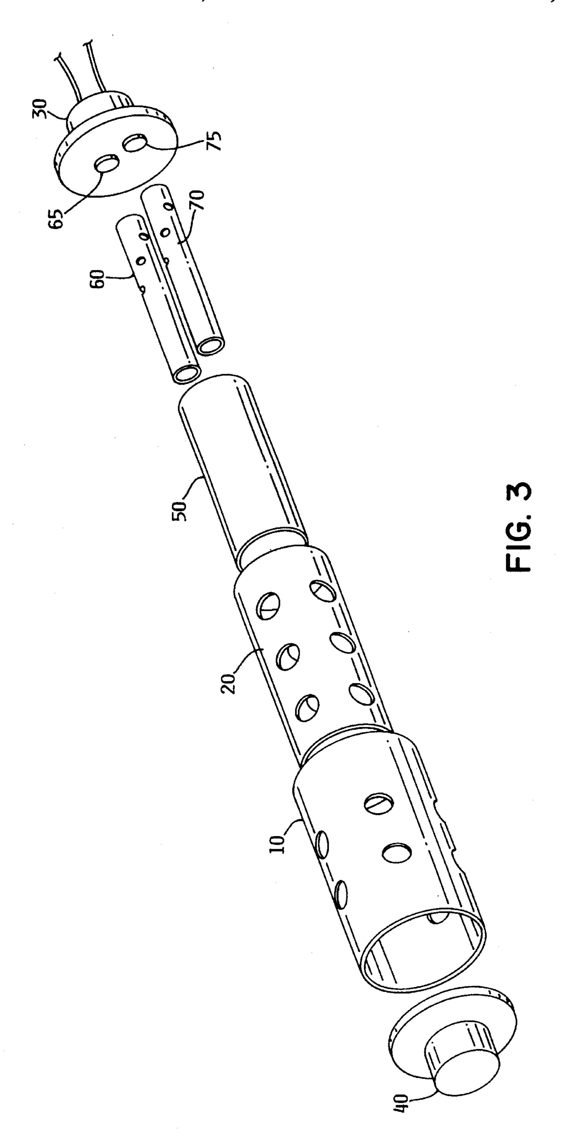
The present invention relates to a gas detector for measuring the concentrations and presence of unwanted or 5 combustible gases so that an alarm can be given when excessive concentrations of such gases are measured. More particularly, the invention relates to a ruggedized construction for a gas detector which houses a gas chamber and an infrared source and sensor for directing infrared radiation through the chamber to the sensor.
